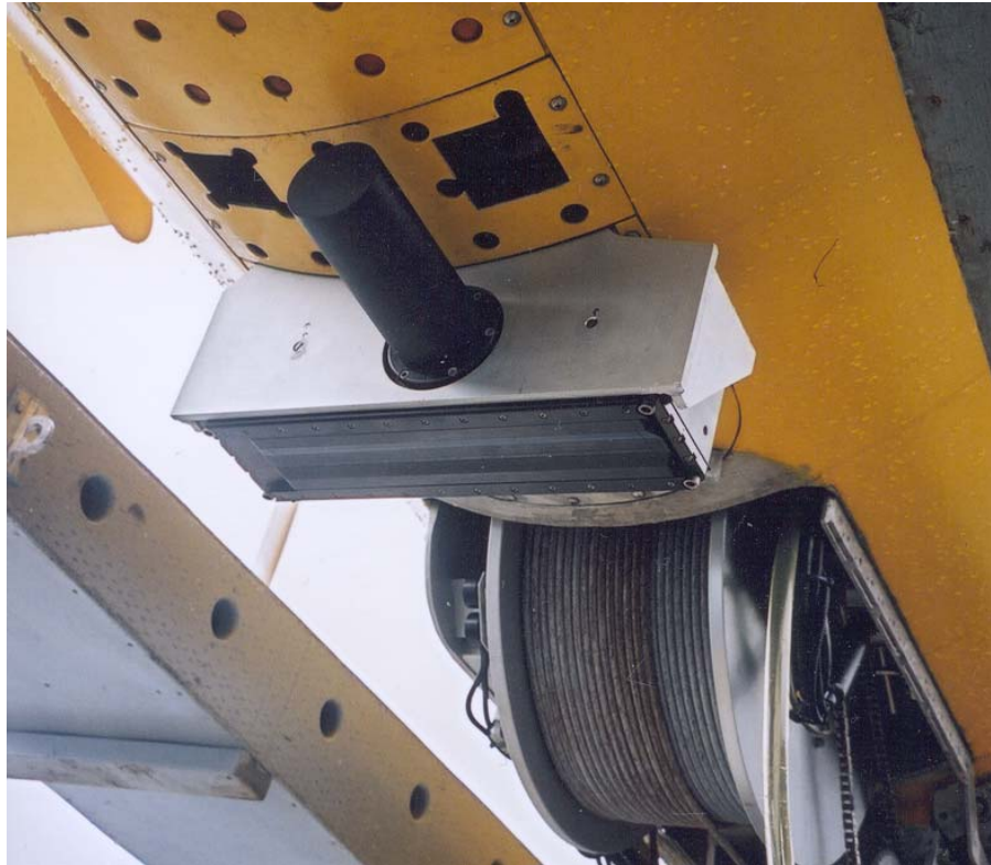
Figure 2 Photograph of the Reson 8125 transducer mounted on the underside of the Dorado vehicle, just forward of the towfish winch assembly in the keel. The black cylinder projecting forward is the transmitter, while the receive array lies behind the black rectangular plate just aft of the projector.
