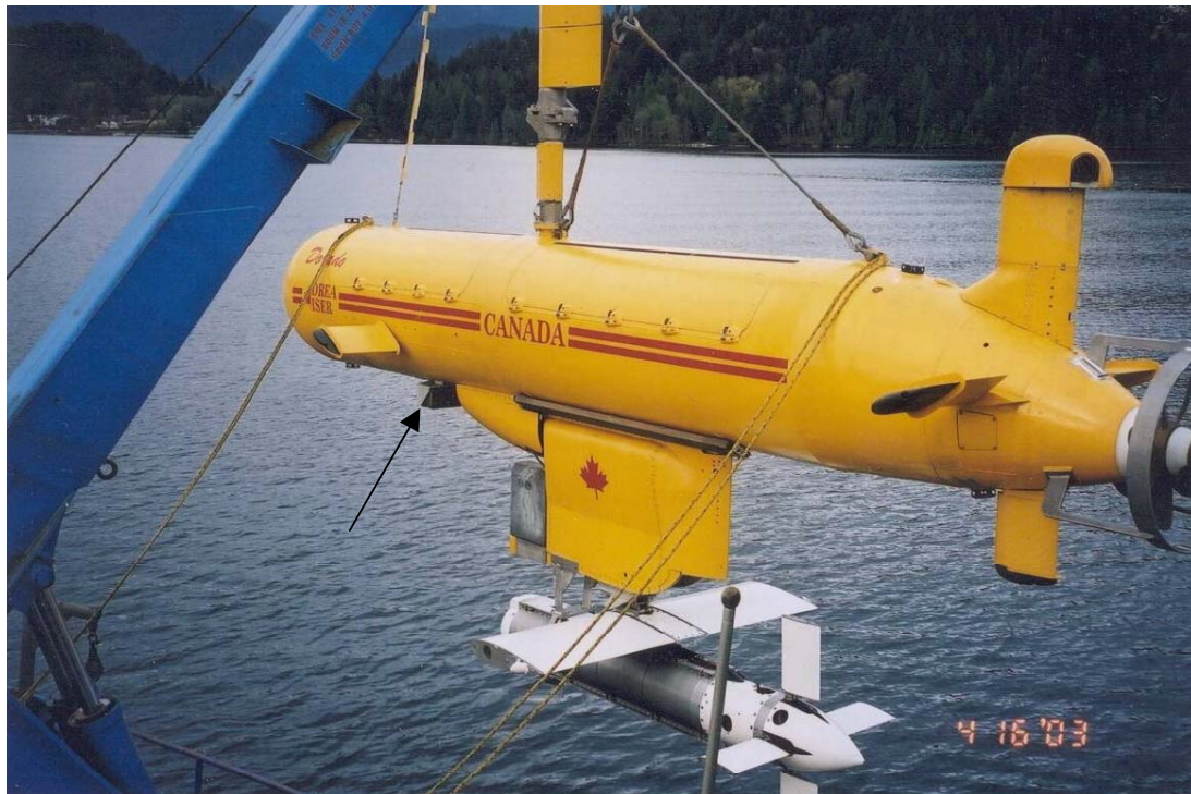
Figure 1 Photograph of the Dorado remote minehunting vehicle being deployed near Vancouver, BC April 16, 2003. Actively-controlled, variable-depth sidescan towfish is attached to the bottom of the keel. Black arrow shows mounting location of sonar head.
