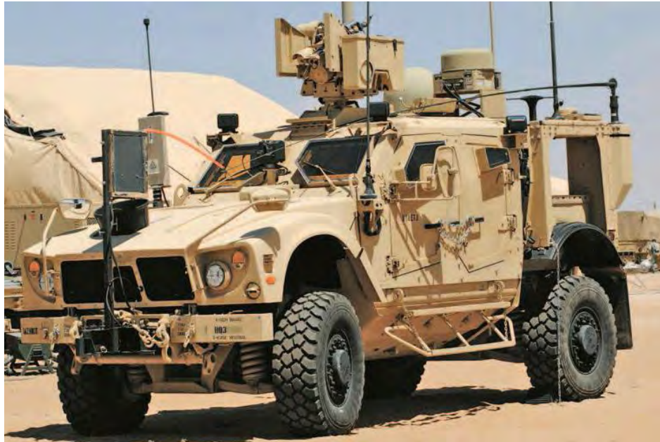
Figure 3. WIN-T Increment 2 POP Equipment Mounted on a Vehicle Source: Army
