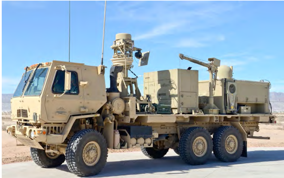
Figure 2. WIN-T Increment 2 TCN Equipment Mounted on a Vehicle Source: PEO C3T Officials
