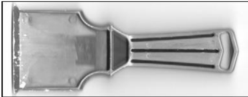
Fig. 4 Plastic Klean Strip high-density polyethylene scraper
