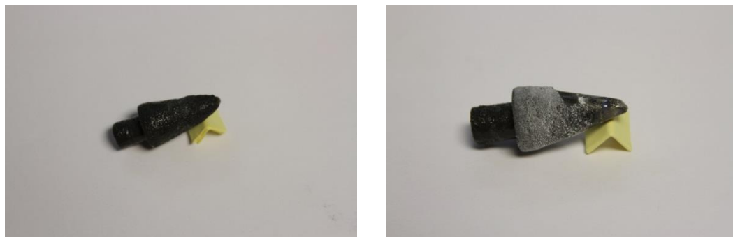
Fig. 10 Pre-test (left) and post-test (right) images of Mo-Si-B coated ZrB 2 -30 vol% SiC cone after a 20-minute ICP torch test.
