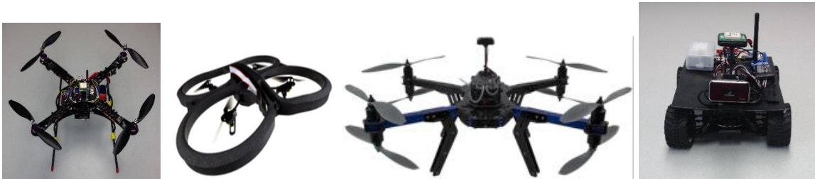
Figure 9: Aducopter, Parrot AR. Drone 2.0, and Adurover used in the testbed
