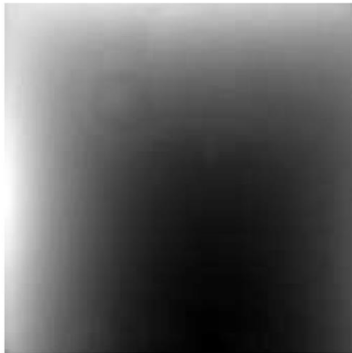
Figure 2. Example temperature distribution produced from IR camera during heat transfer experiment.
