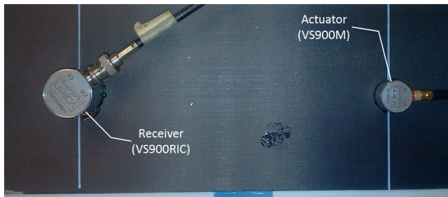
Figure 9. Experimental setup used for investigating stacked delaminations.
