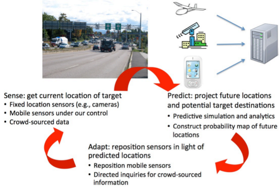
Figure 1.1: DDDAS processing loop for vehicle tracking.
