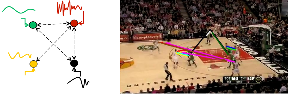
Figure 8: Finding causal interactions as a graph identification problem. Left: Representation of this sequence as a graph, where each node represents the time series associated with the position of each player and the links are vector regressive models. Causal interactions exist when one of the time series can be explained as a combination of past values of the others. Right: Application of these ideas to the problem of finding causally interacting players in a basketball game.
