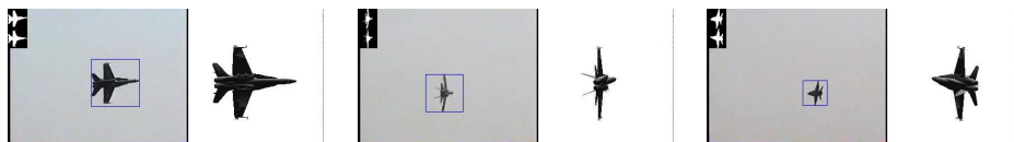
Figure 4: Using a Hammerstein/Wiener system to achieve sustained tracking in the presence of appearance changes. The left and right portions of each frame show the actual and predicted target appearance, with their correlation displayed in the top left corner.
