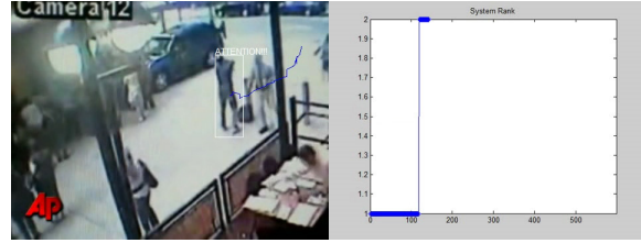
Figure 6: . Fast event detection. The jump in the rank of the Hankel matrix indicates a change in dynamics as the suspect of a 2010 bombing attack in New York City stops to remove his sweater.
