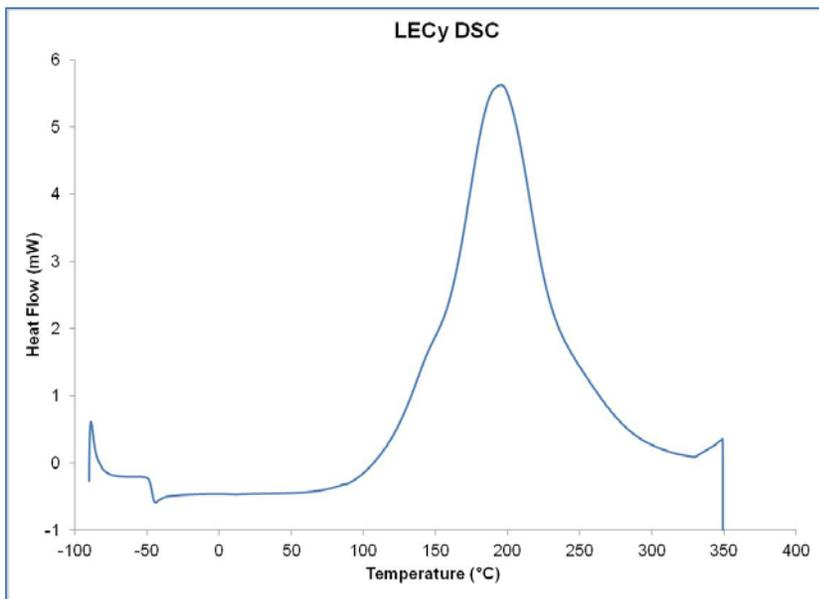
Impurities, such as aryl phenols and transition metals, catalyze cyclotrimerization and lowers the peak of the cure exotherm temperature thereby narrowing the processing “window.”
