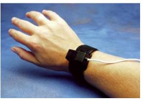
BioPac Systems Tri-Axial Accelerometer
