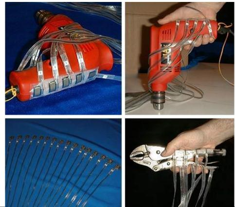
Cable Length: Each wire is 20 inches long with all wires gathering to a IDC connector which attaches to a 6 ft. Ribbon cable extension that plugs into the interface module.
