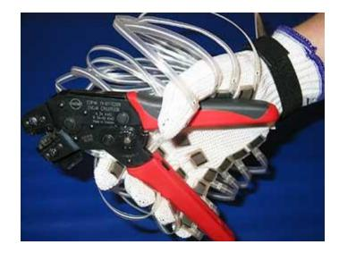
Twenty and twenty-four sensors are used in the standard configurations that results in a sampling rate of over 100 Hz. They are calibrated with a known load in a calibration jig. Variation coefficient (which is the standard deviation expressed as a percentage) is within acceptable quality control range of  $\pm$  10%
