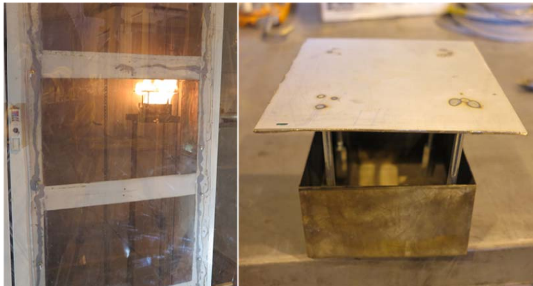
Figure 5. (Left) Heptane fire in test 16. (Right) Picture of the fuel pan with obstructing panel approximately 50 mm above pan edge.
