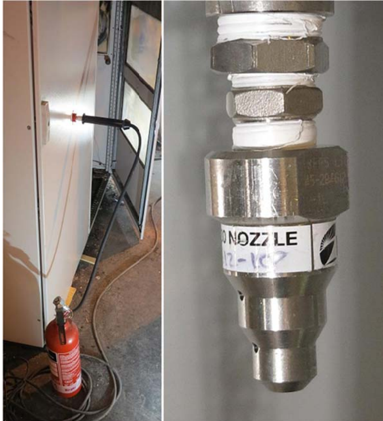
Figure 7. (Left) Hand held CO 2 extinguisher (2 kg) connected to cabinet through NATO coupling. (Right) NOVEC 1230 (180°) nozzle used for all NOVEC 1230 and nitrogen fire suppression tests.
