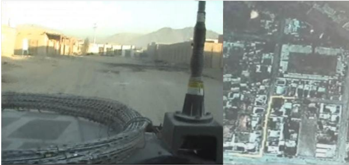
Figure A.1: Screenshot of the first EFIT prototype with ground vehicle video of Afghanistan beside aerial imagery showing the moving position of the camera (yellow line).
