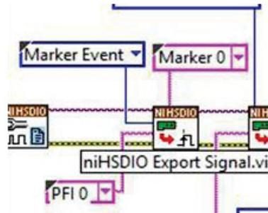
**Figure 4-40: HSDIO event signal output and configuration**
