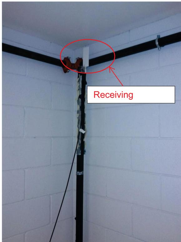
*Figure 4-26: Receiving antenna placed in the corner of the room*
