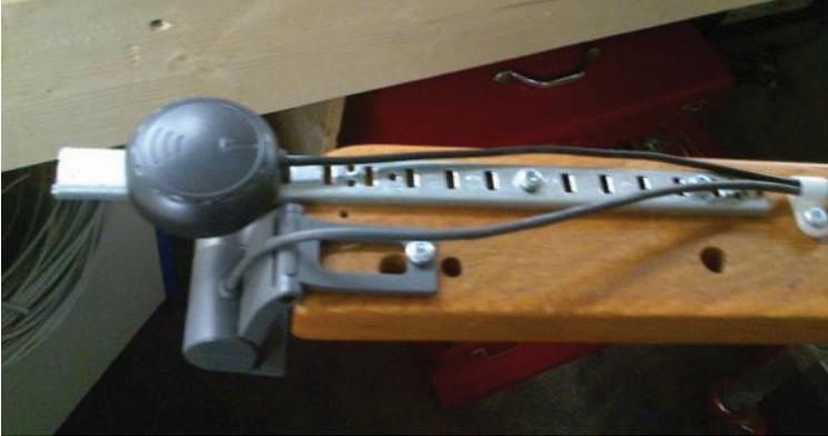
Figure 4-12 Close-up of the receiver antenna and the web-cam
