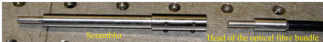
Figure 32: Scrambler device place at the entrance of the optical fibre bundle.
