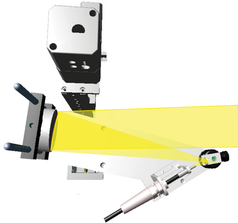
Figure 30: Setup with the tilt f/4 50 mm spherical mirror mounted on the scanner.
