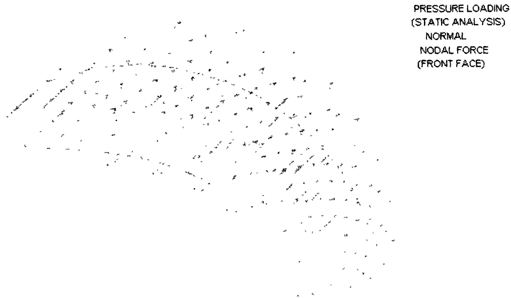
Figure 5.14: Normal Force Vectors at Front Face of P5363 Propeller Blade
