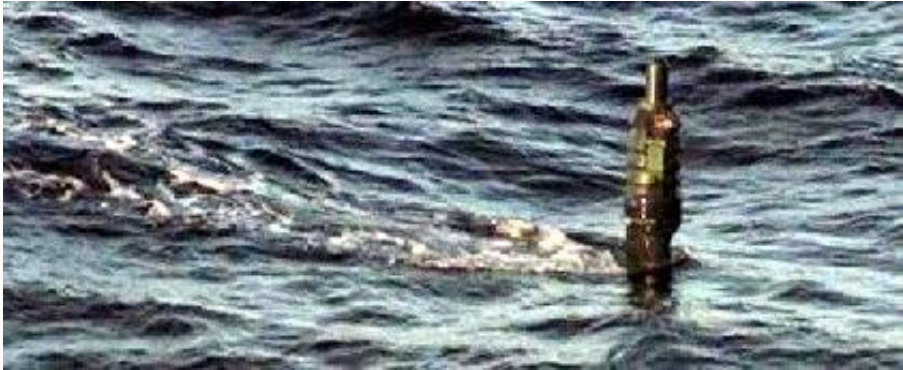
Figure 11. Photonics mast array on a Virginia-Class submarine
