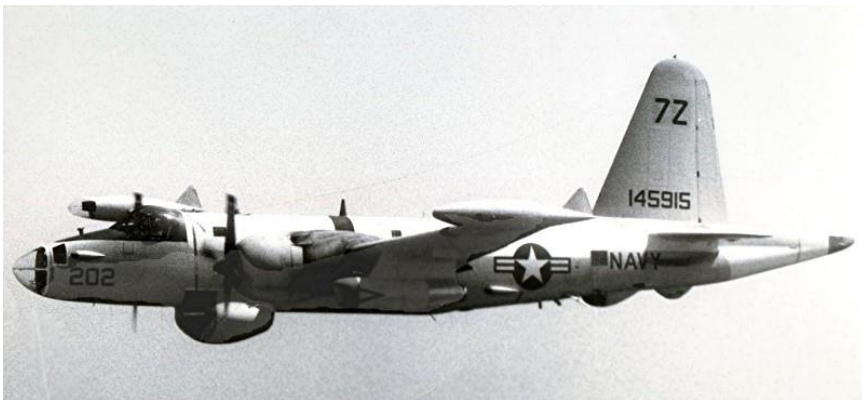
Figure 12. P2V-7 aircraft with AN/APS-20 radome on its underside
