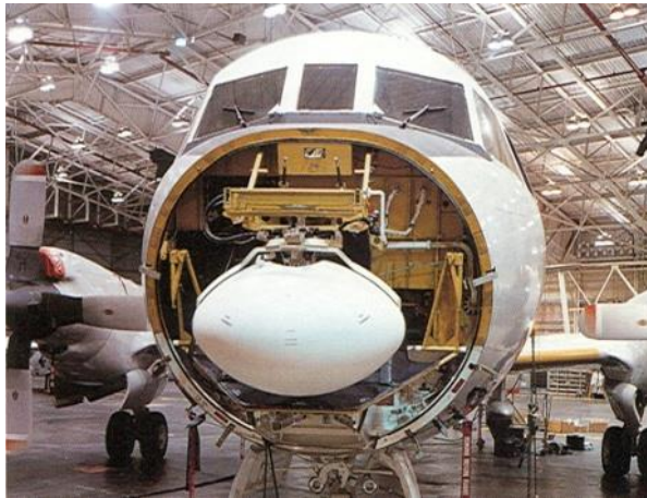
Figure 17. AN/APS-137 antenna in nose of P-3C Update III Aircraft
