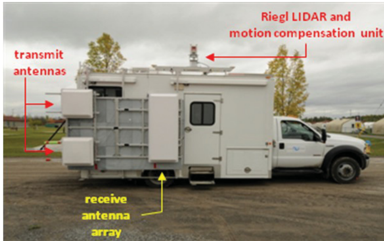
Figure 1. 3-D through-wall SAR system.
