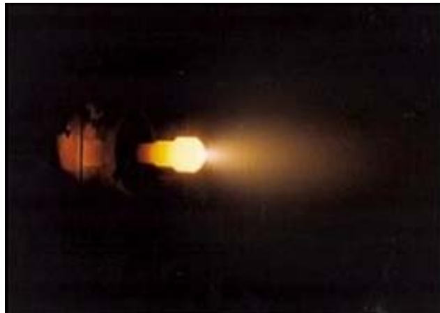
Aerojet MR-510 Arcjet Propellant: Hydrazine Thrust: 250 mN Isp: 585 sec
