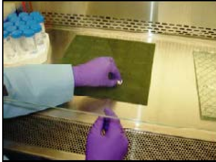
Figure 3. Example of surface sampling on a panel using a wipe 1 .
