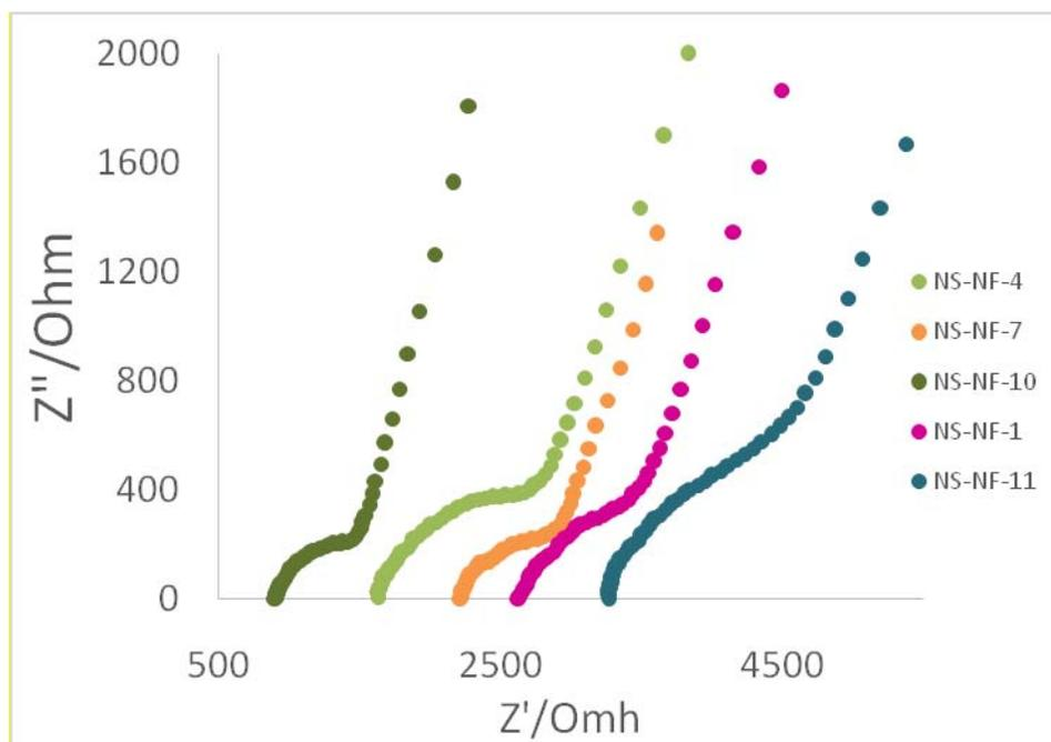
**Figure 22:** Electric conductivity measurements of PCL nanofibers coated with unmodified hydrogel (NS-NF-1), with sulfonate modified hydrogel (NS-NF-4), with carboxylate modified hydrogel (NS-NF-7), with phosphate-modified hydrogel (NS-NF-10), and without coating (control).
