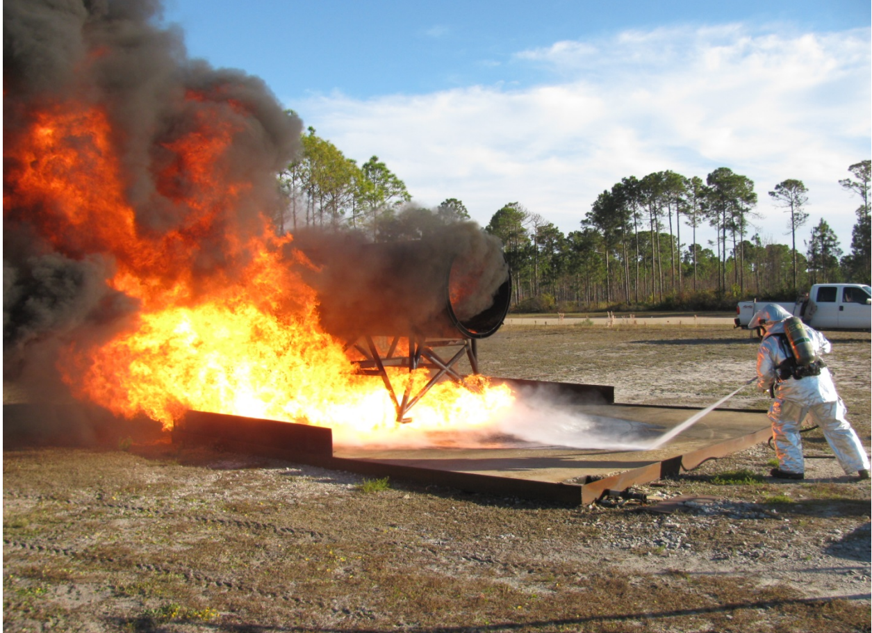
Figure 13. Rear Engine Fire Using a 0.165-in Stoneage Nozzle at 2100 psi (Note the burning fuel being pushed towards the rear of the test structure by the force of the agent stream.)
