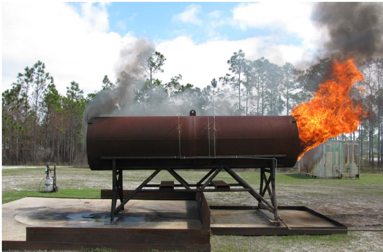
Figure 6. F-100 Nacelle Mockup during Pre-Burn Phase of a Rear Engine Fire Test
