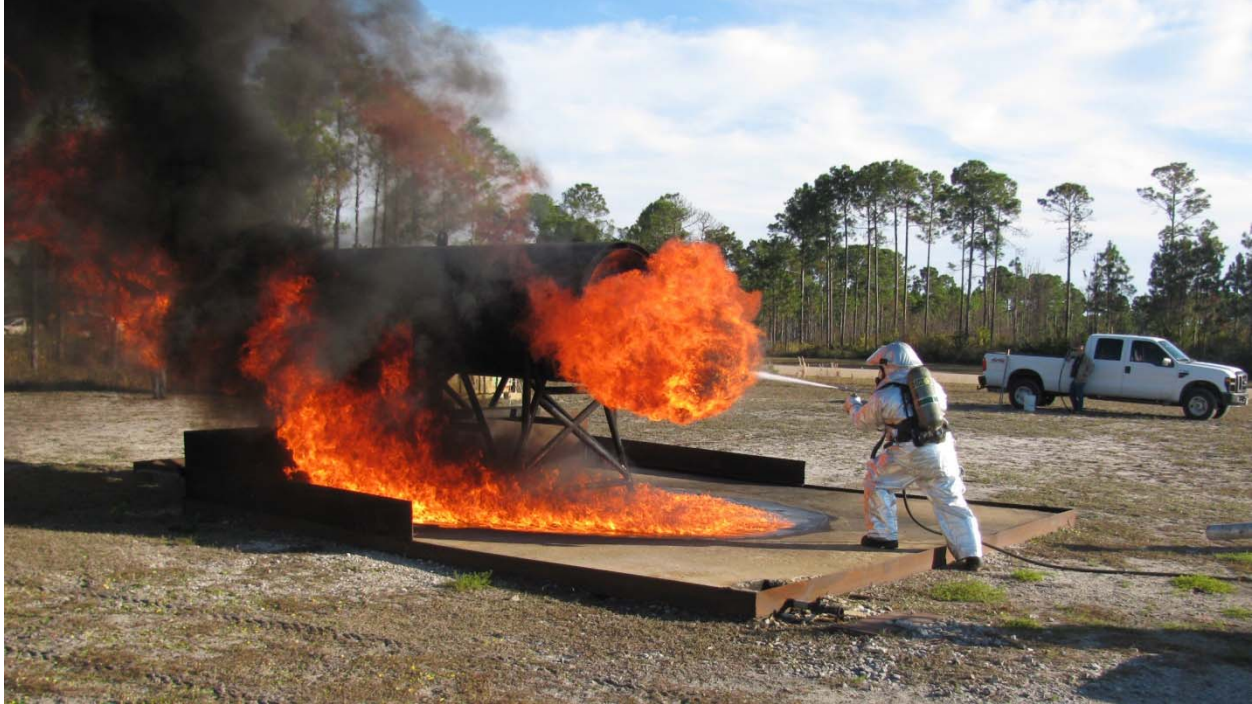
Figure 7. Firefighter Applying Agent during a Rear Engine Fire Test
