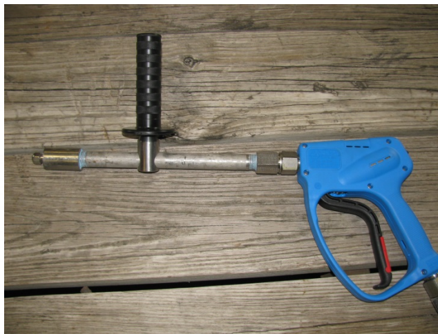
Figure 10. StoneAge Attack Tip Nozzle (Left- illustration of the StoneAge Attack Tip nozzle. Right- Photograph of a StoneAge Attack Tip nozzle attached to a trigger gun.)
