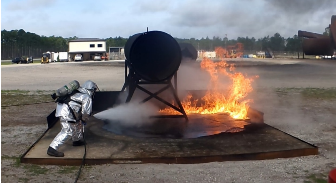
Figure 14. Pool Fire Using a 0.243-in StoneAge Nozzle at 1500 psi (Notice that the ground fire is largely suppressed; however, the extinguisher ran out of agent before the fire was completely extinguished.)
