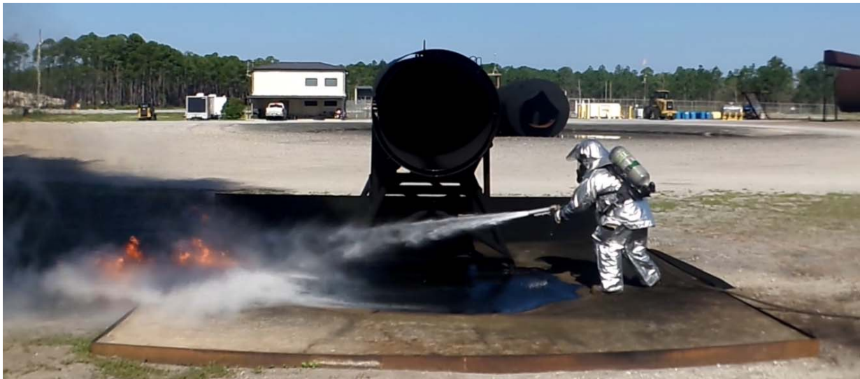
Figure 16. Extinguishing a Pool Fire Fire Using a 0.230-in Rosenbauer Nozzle at 1050 psi
