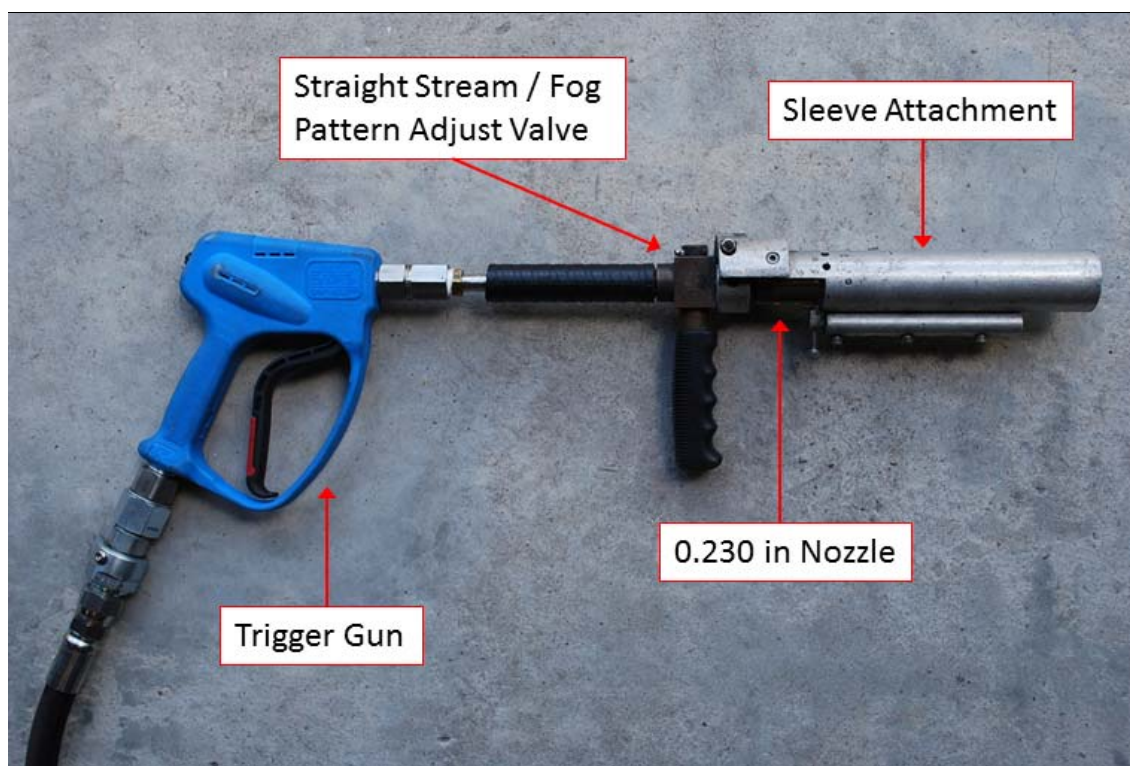
Figure 15. Rosenbauer Nozzle and Trigger Gun with Custom-made Sleeve Attachment
