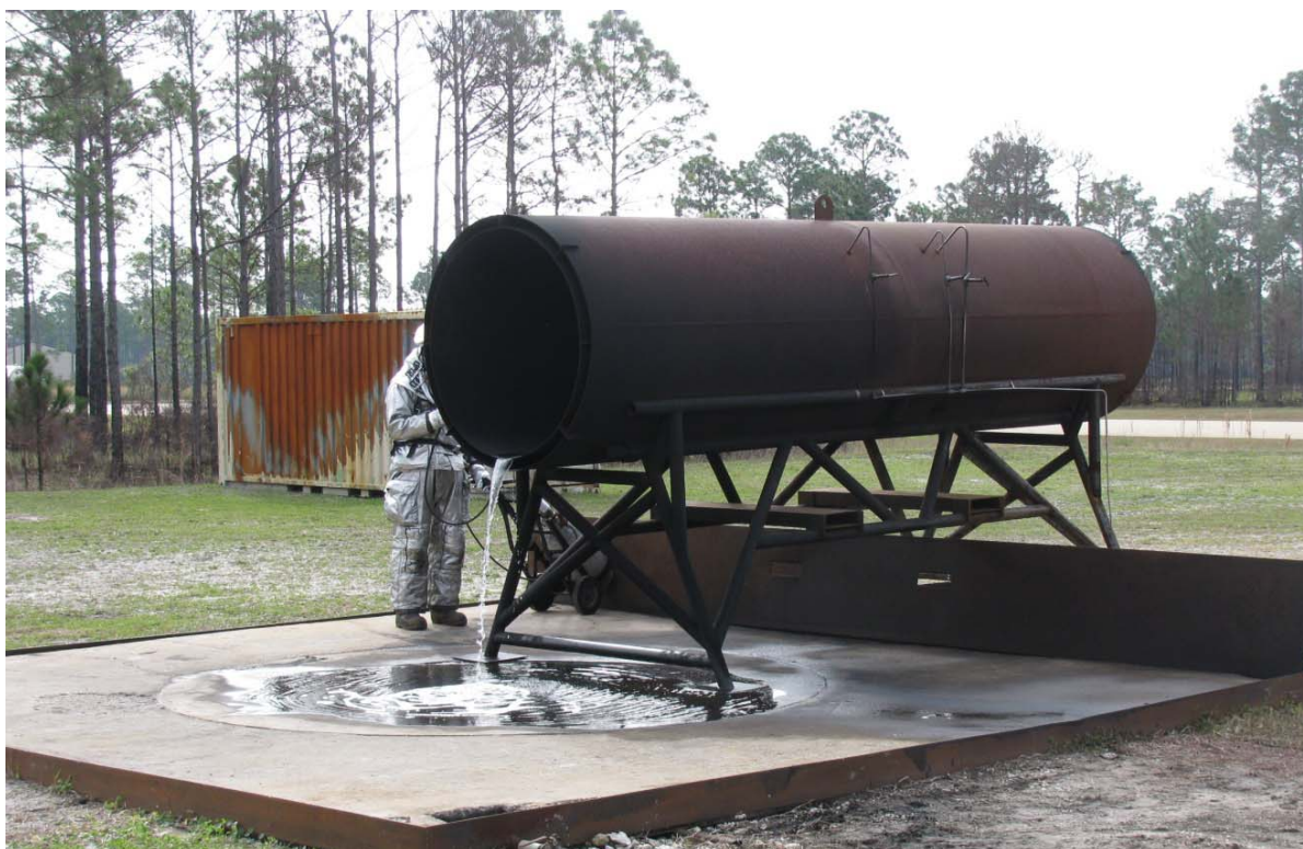
Figure 5. F-100 Engine Nacelle Mock-Up (In This Photo, Fuel Is Flowing through the Nacelle in Preparation for a Rear Engine Test.)
