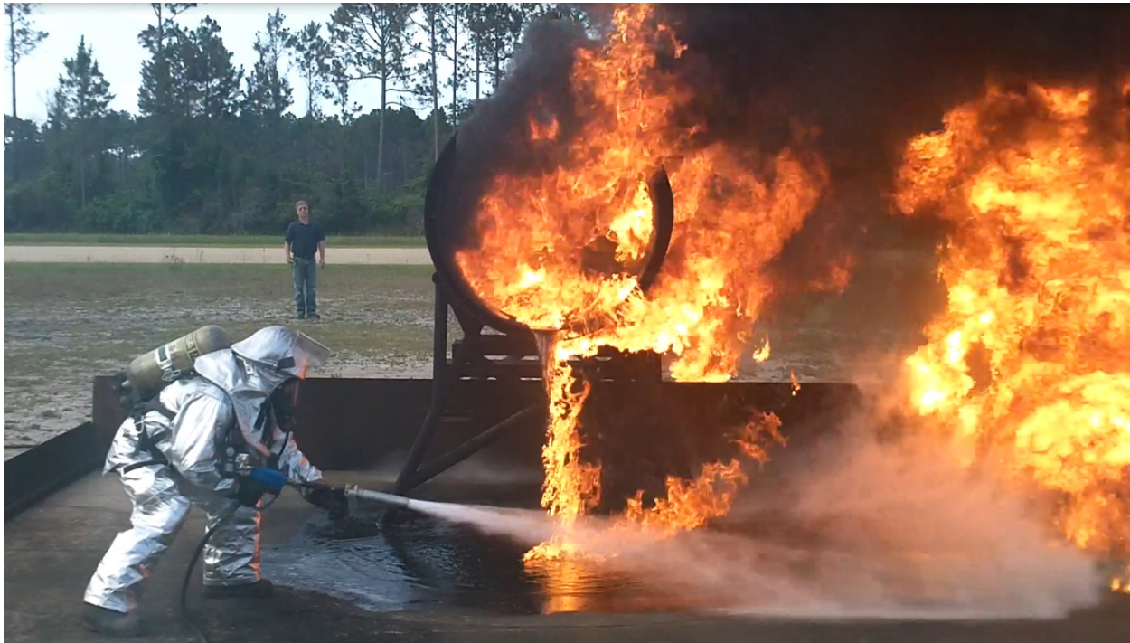
Figure 17. Rear Engine Fire Using a 0.230-in Rosenbauer Nozzle at 1050 psi
