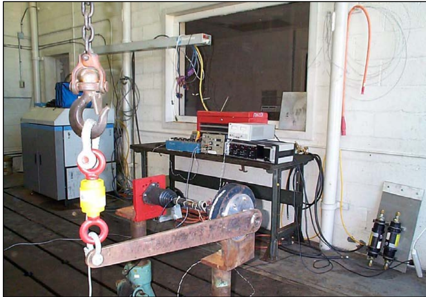
Figure 4. Torque calibration of a high mobility multipurpose wheeled vehicle (HMMWV) axle half shaft.
