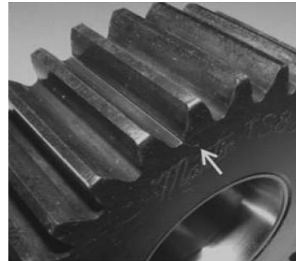
Figure 11. 4.3 mm manually made tooth crack in planet gear
