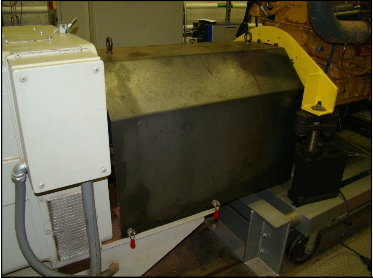
Figure 7. Shaft guard installed.
