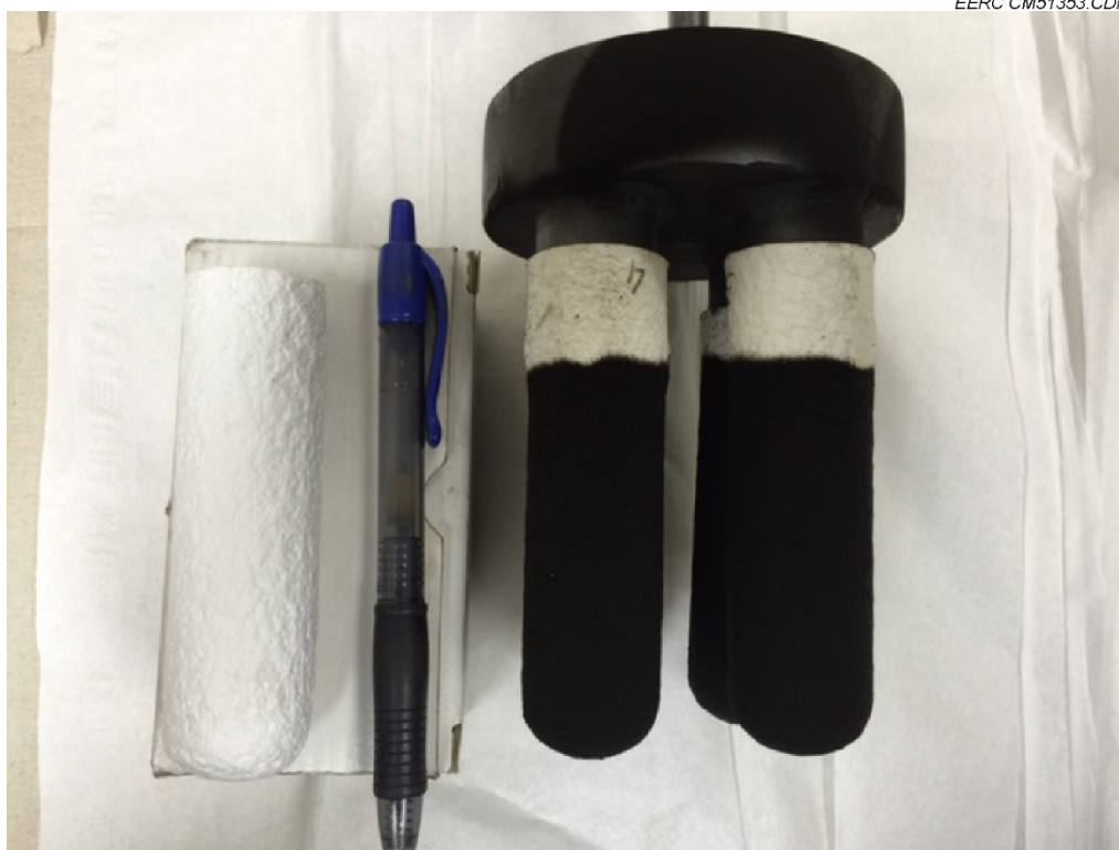
Figure 22. Typical appearance of an exposed set of tar-sampling particulate filters.
