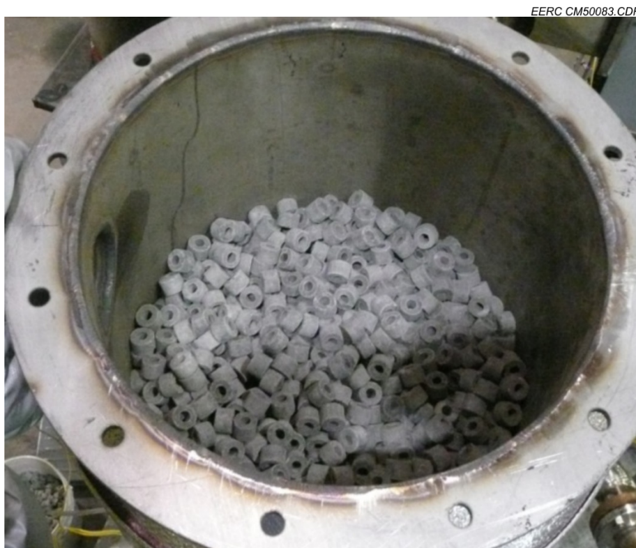
Figure 12. View into reforming reactor after catalyst filling.
