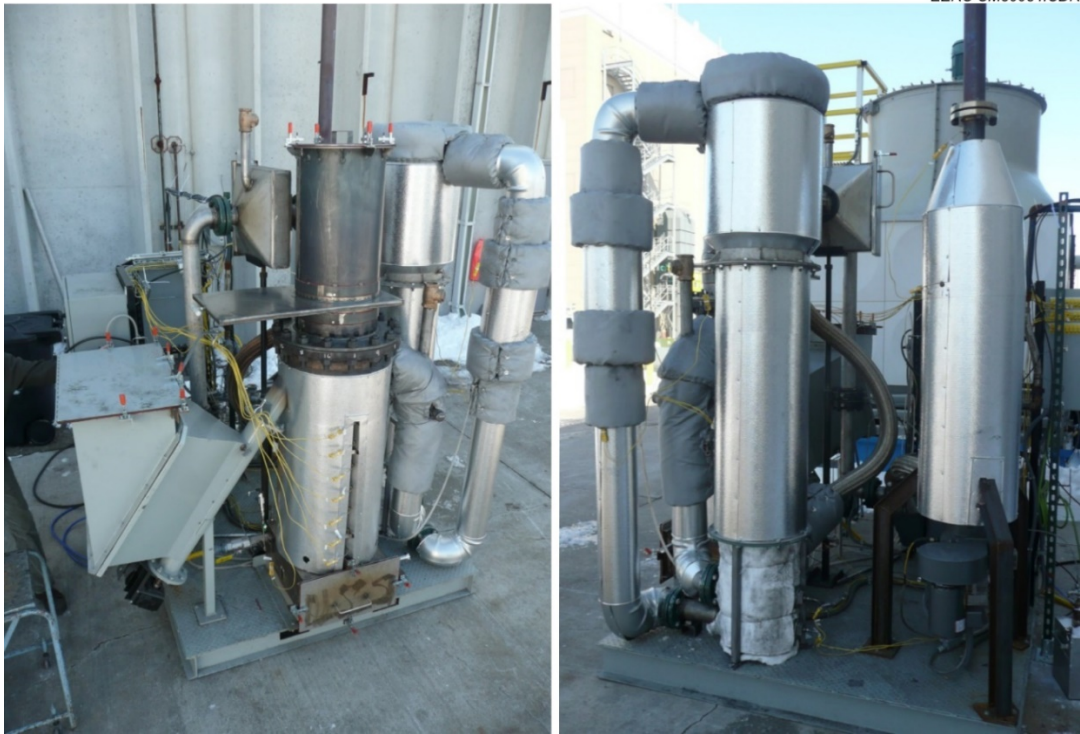
Figure 9. Photographs of the skid-mounted prototype gasification and cleanup system.
