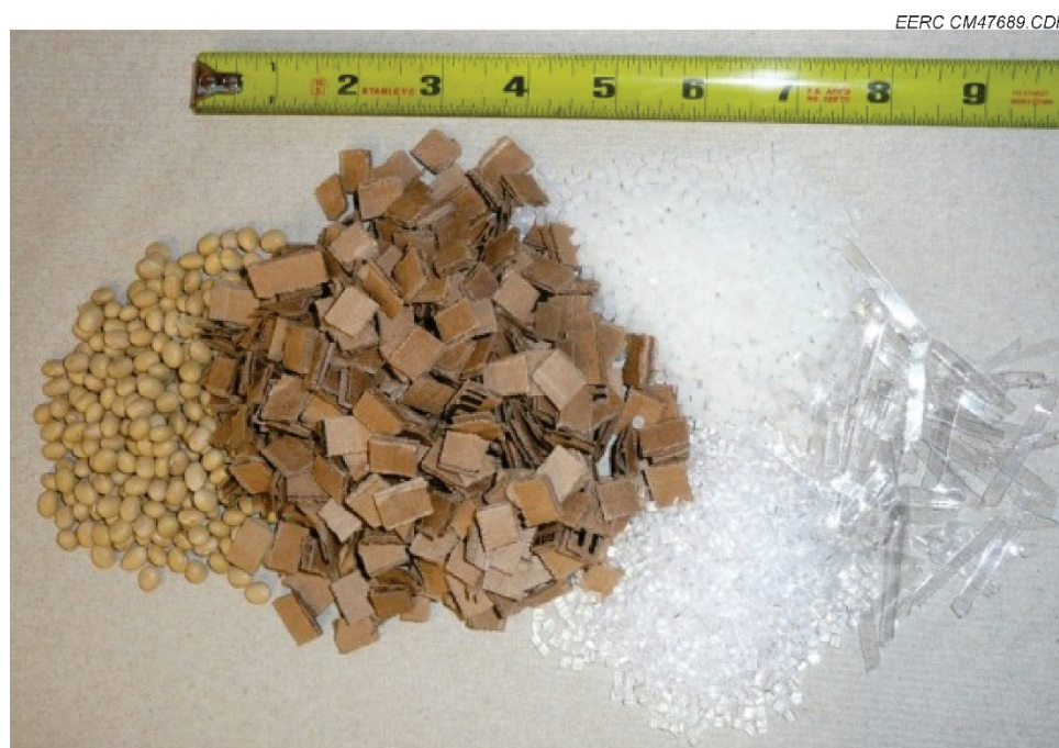
Figure 6. Tested fuel mixture components, from left: soybeans (shown dry), cardboard, polystyrene and polyethylene, and PVC film.
