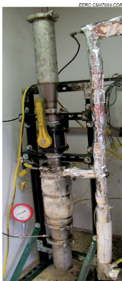
Figure 5. Laboratory countercurrent gasifier.
