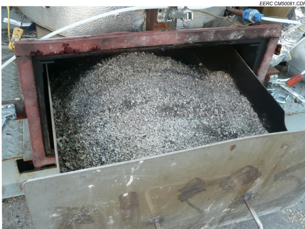
Figure 24. Typical ash collection from the test fuel mixture.
