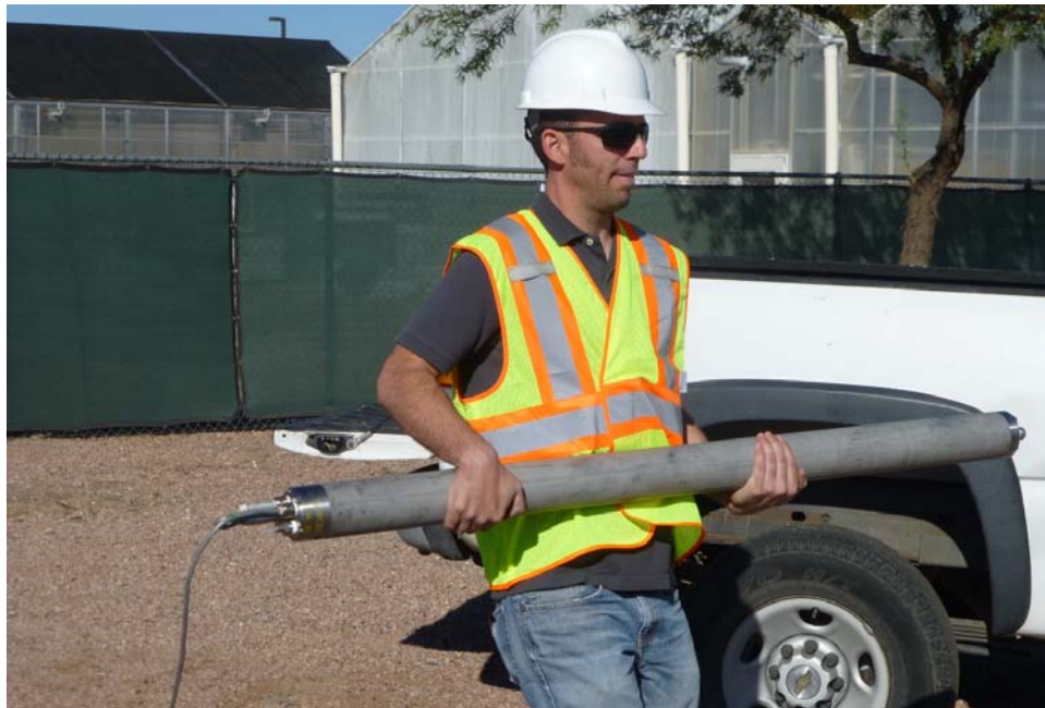
Figure 9. IS2 sampler with peristaltic pump in its watertight shell. Ports in the shell provide fluid inlets, gas pressure relief, and electrical connections.
