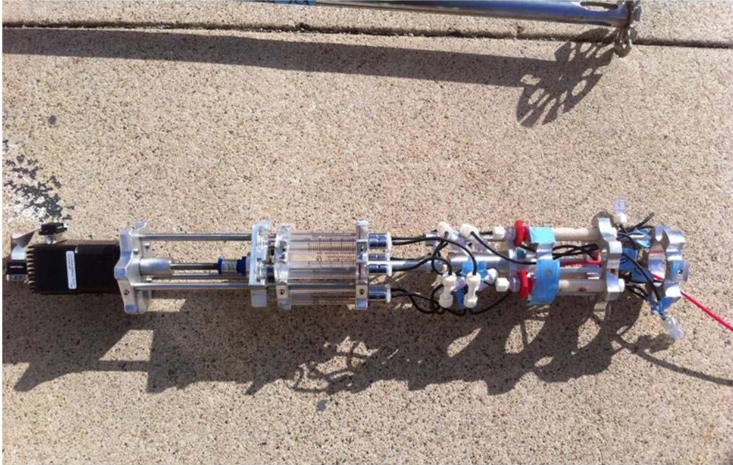
Figure 14. Field-prepared IS2 sampler with reciprocating syringe pump.
