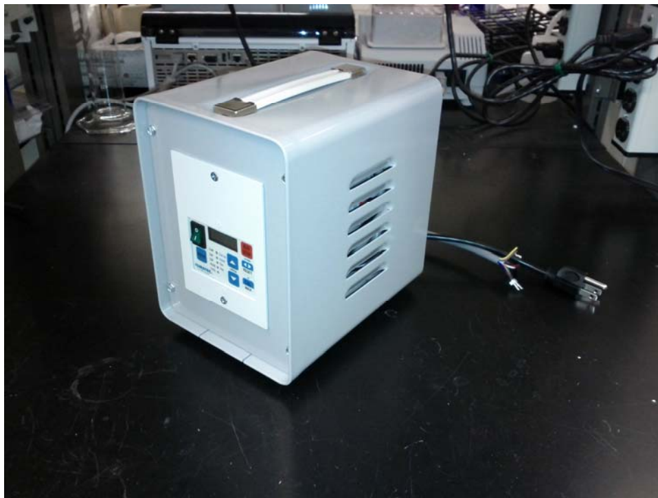
Figure 10. IS2 peristaltic pump control unit.
