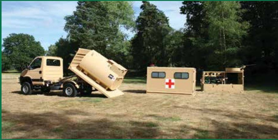
FIGURE 6. CAMELEON DE-MOUNTABLE FUEL BOWSER WITH AMBULANCE AND PATROL MODULE IN REAR
