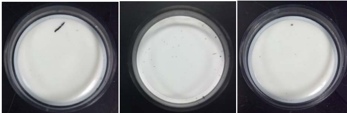
Figure 1. Examples of filter monitors with large visible particulates
