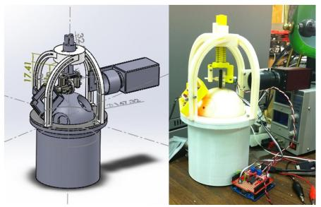
lattice of spring-loaded interchangeable scatterers (Figure 4b). Compressed air flows into the Kugel base (Figure 4c), evenly fluidizes the Kugel through an air distributer.
