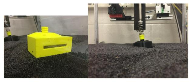
A smaller granular bed was fluidized with pressurized air that was activated via automation with this custom printed flow valve that had internal solenoid valve actuation.
