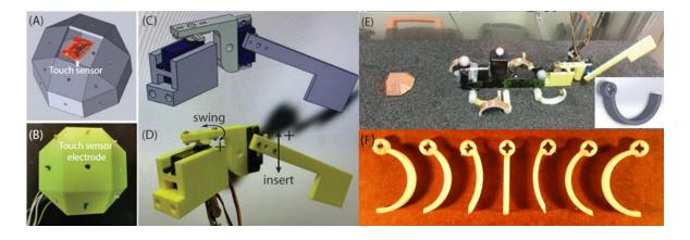
Using the automated terrain creation and robot testing system [2], we collected ~3000 runs of a hexapedal robot locomotion in a trackway filled with ~1mm poppy seeds (the "sand") with a single "boulder" embedded in. We found that the robot interaction with each single boulder can be modeled as a scattering event.
