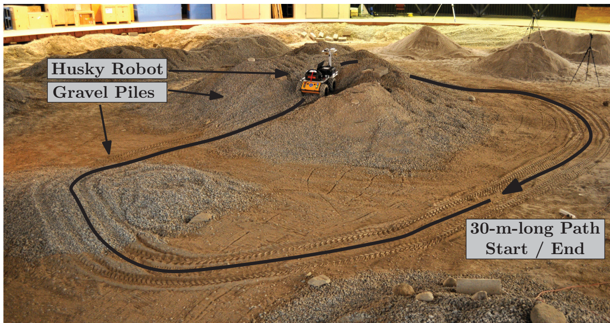
Figure 7: The first and second experiments were conducted inside the University of Toronto Institute for Aerospace Studies (UTIAS) MarsDome on gravel, sand, and loose dirt. The 30-m-long path, shown here, was used for the first experiment. In all experiments, the nominal unicycle model used in our LB-NMPC algorithm included no prior information on wheel-terrain interactions or robot dynamics.
