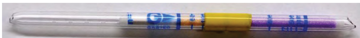
Figure 4-7: \text{NH}_3 concentration measured using a Gastec tube during suppression of a diesel fire using a StatX aerosol unit inside the UW Burn Room (564 seconds) 5
