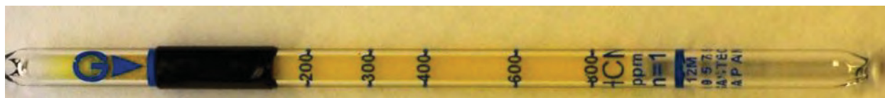
Figure 4-6: HCN concentration measured using a Gastec tube during suppression of a diesel fire using a StatX aerosol unit inside the UW Burn Room (444 seconds) 4
