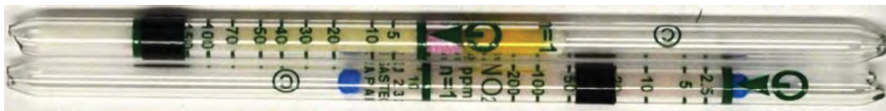
Figure 4-38: NO x concentrations measured using Gastec sampling tubes during release of a StatX unit in a cold test compartment with no fire (Test 3, 170 seconds)
