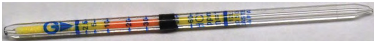
Figure 4-49: HCN concentrations measured using Gastec sampling tubes during release of a DSPA 5-4 unit into a cold compartment with no fire (Test 3, 297 seconds)
