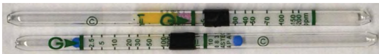
Figure 4-15: NO and NO 2 concentrations measured using Gastec tubes during suppression of an obstructed bilge fire using a StatX aerosol unit (770 seconds)
