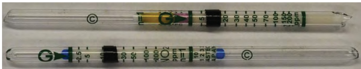
Figure 4-24: NO and NO 2 concentrations measured using Gastec tubes during suppression of a wood crib fire using a Stat X aerosol unit (600 seconds)
