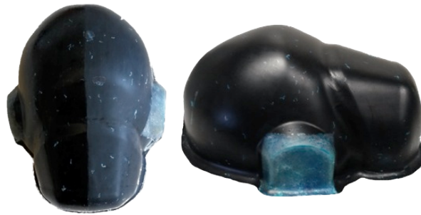
Figure 3.16 Prototype parts made at the Oxford Silk Group: silk reinforced composite outer shell of a crash helmet.
