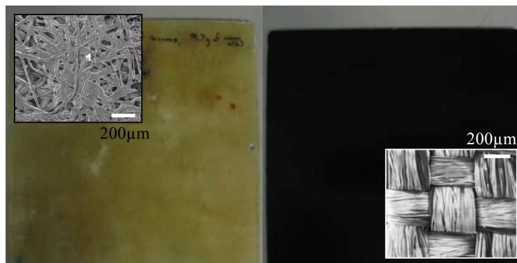
Figure 3.12 Silk composite laminates: Nonwoven mat (left) and biaxial woven fabric (right) reinforcements.
