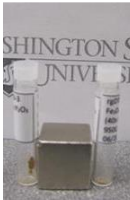
Figure 113. Images of \text{Fe}_3\text{O}_4/\text{Eu}:\text{Y}_2\text{O}_3 core/shell nanoparticles in the presence of a magnet. Precursor (left), heated to 600 °C and 700 °C (center), and heated to 800 °C and 950 °C (right). All samples are magnetic, except the one heated to 950 °C.
