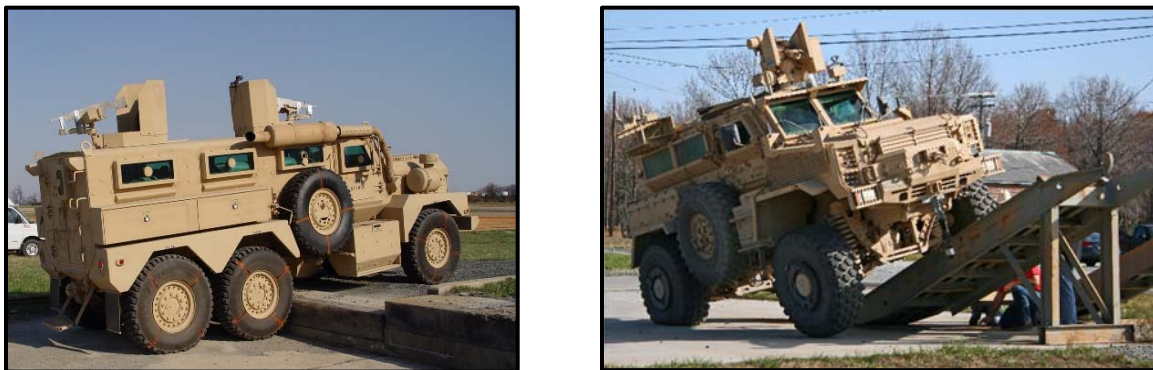
Figure 10. Vertical step and RTI fixture checking tire clearance.
