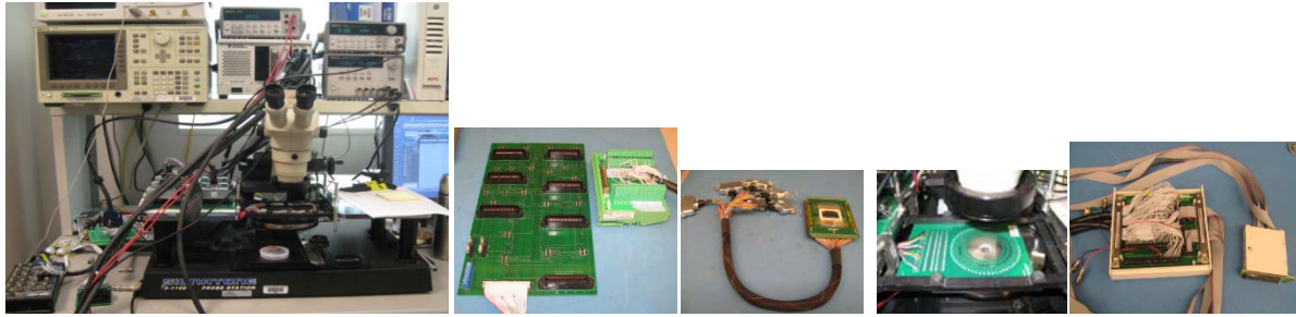
Figure 21. From left to right: Completed array test station; custom decoder board, 300 pin wafer probe card; 10 x 10 probe card; PXI matrix interface board
