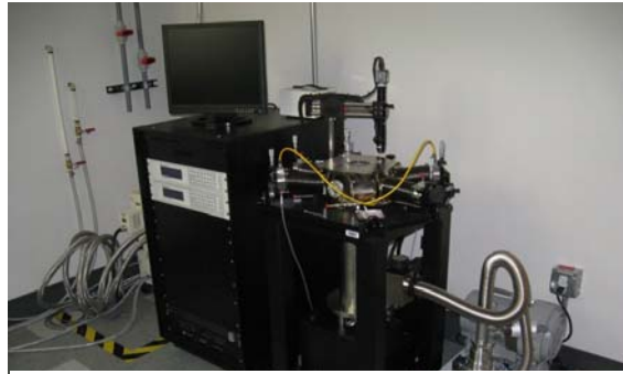
Figure 20. Cold temperature probe station
