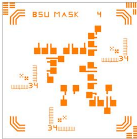
Figure 90. BEOL mask 4, top electrode definition
