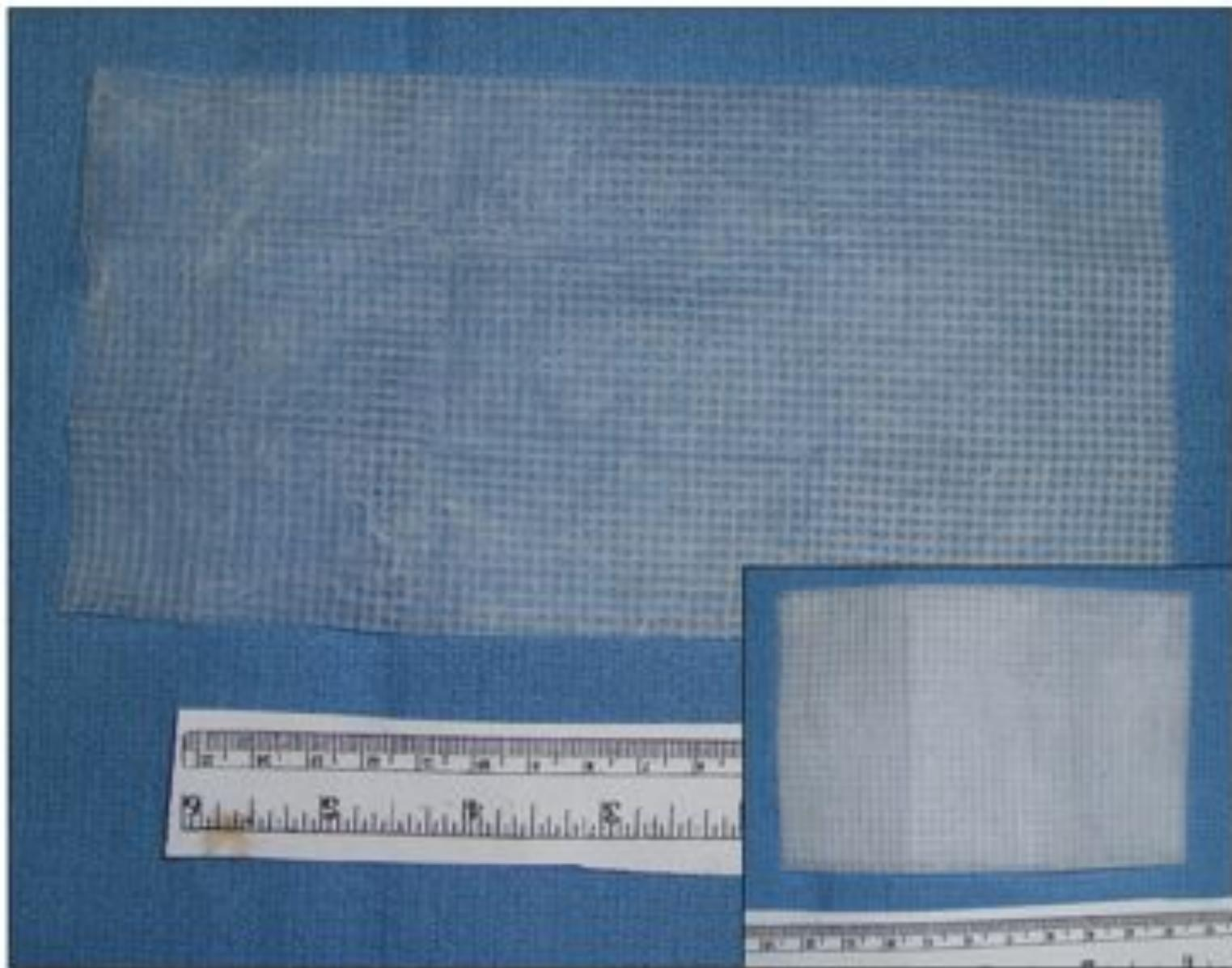
Fig. 1. PCL mesh (test bandage for NEDED project). Single ply, ~20 x 10 cm (8 x 4 in). Inset: folded into thirds, ~10 x 6.7 cm (4 x 2.7 in), as used *in vivo*. Bandage wt ~0.5 g.
