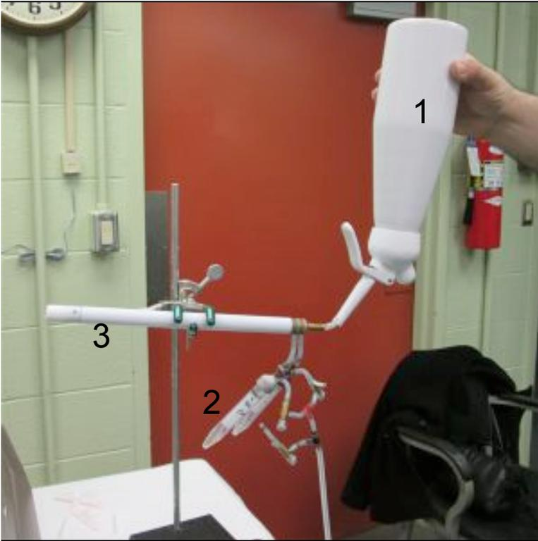
Figure 3, swine 211. Injection apparatus. (1) Commercial creamer container for alginate. (2) Conical tube containing biologics. (3) Injector nozzle.
