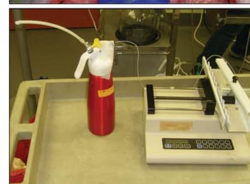
Fig. 3: Alginate Foam Injecting Equipment.
