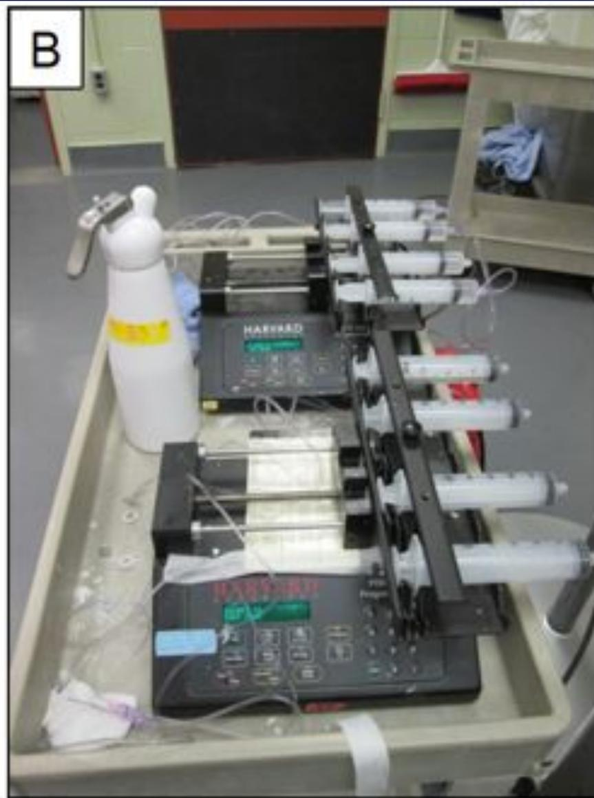
Alginate Reservoir And  $\text{CaCl}_2$  Pumps
