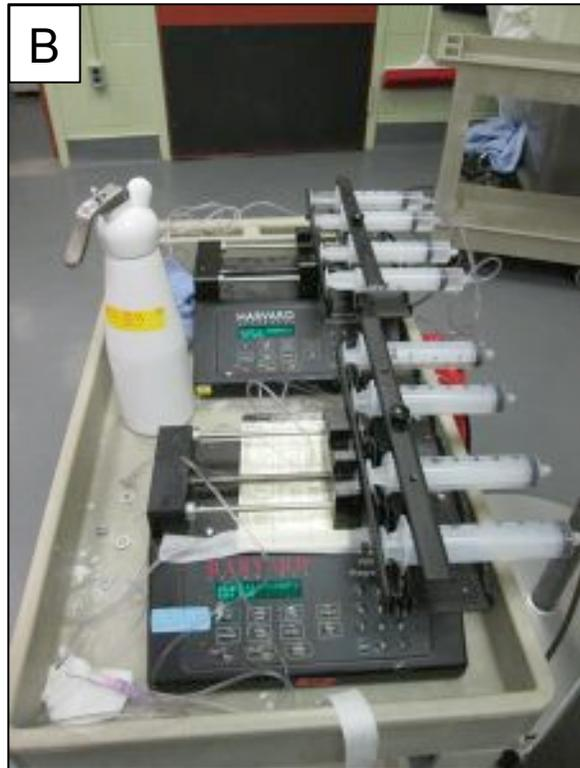
Figure 3, swine 203. Foam injector set-up. (A) Canister. (B) Two syringe pump set-ups (four syringes per pump, for parallel injection of calcium chloride).
