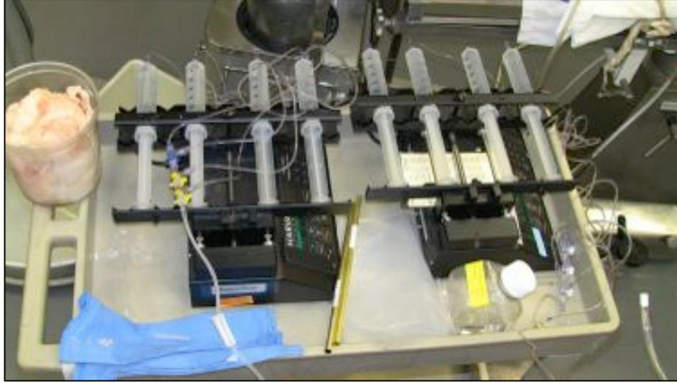
Fig. 1, swine 200. Set-up for syringe pumps for infusion of  $\text{CaCl}_2$  solution into the alginate foam injection system. Four pumps (each using a 50 cc syringe) are used in parallel during each injection. Canister of *ex vivo* injected foam is sitting at left.
