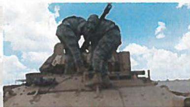
**Task:** Install an M242 25mm Barrel on the M242 Gun on a BFV; Two Soldier Task
