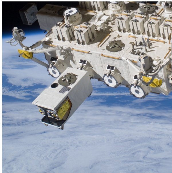
Figure 2000s.7.5 - The gold-blanketed RAIDS experiment views the atmosphere aftward from the open end of the HREP while attached to the Japanese Experiment Module Exposed Facility (JEM-EF) (credit: NASA).
