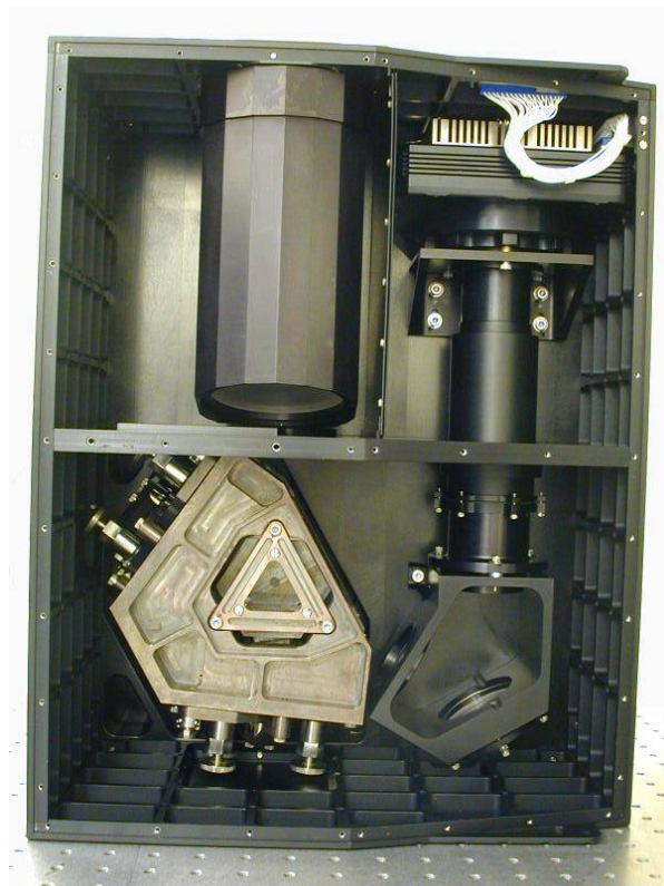
Figure 2000s.5.1 - SHIMMER-MIDDECK optics assembly. From the top left counterclockwise: Telescope, SHS interferometer mounted in a VascoMax steel cage, relay optics, CCD camera (credit: This figure first appeared in Cardon et al., 2003).
