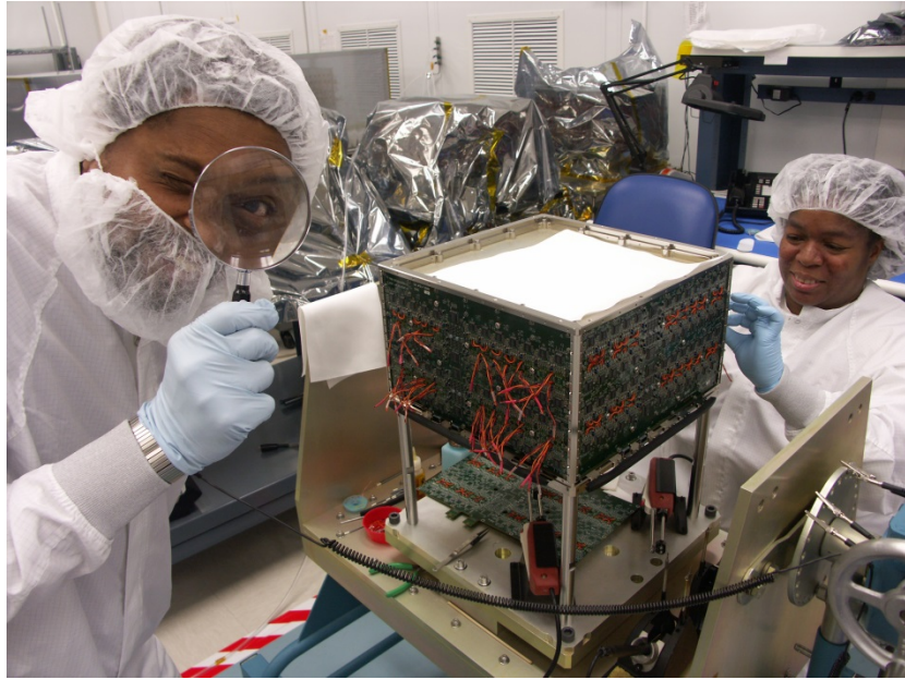
Figure 2000s.1.1. Photo of one of the 19 calorimeter modules (16 for flight, 3 spare) during assembly in the clean room at NRL. James Lee (left, ATK, Inc.) and Mary Johnson-Rambert (NRL/SSD) are attaching the electronic circuits to the four sides of the module. Each calorimeter module weighs about 90 kg. Completed modules are seen in the background in electrostatic bags (credit: NRL).
