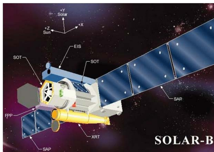
Figure 2000s.4.1 – The Hinode (Solar-B) spacecraft. The EIS spectrometer is shown at the top. The SOT is the white light Solar Optical Telescope, and the XRT is the X-ray Telescope (credit: ISAS/JAXA).
