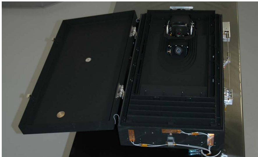
Figure 2000s.3.3 - The Heliospheric Imager (HI) package of the SECCHI instrument. The HI was mounted on the side of the spacecraft and looks along the Sun-Earth line. Two telescopes are at the far end of the package, which has occulters and baffles to block unwanted stray light from entering the apertures. Everything is coated with black paint or some other low-scattering material to reduce the light from the Sun by more than a factor of 10^{-10} . The door which covered the entire box is shown in the deployed configuration. It protected the instrument from dust during the ground operations and launch (credit: NASA/NRL).
