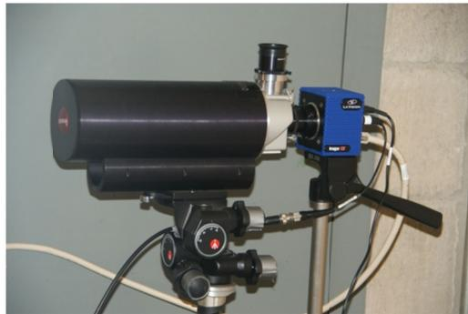
**Figure 6:** The Questar QM-1 catadioptric microscopic lens, attached to the PIV camera.
