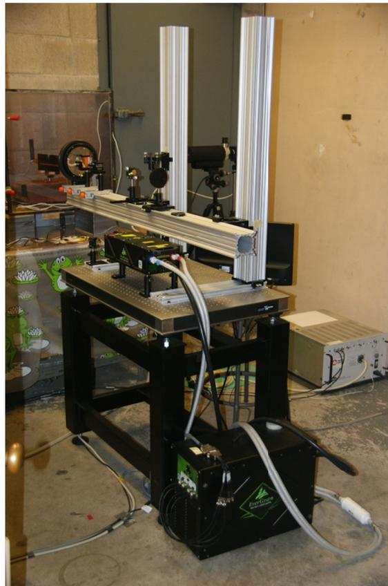
**Figure 5:** The PIV measurement setup, and the high voltage amplifier.
