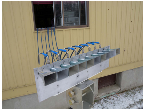
Figure 3: Photograph of the linear array assembled for the time-division MIMO experiment.
