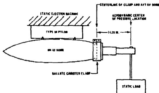
Figure 6. Static load test arrangement
