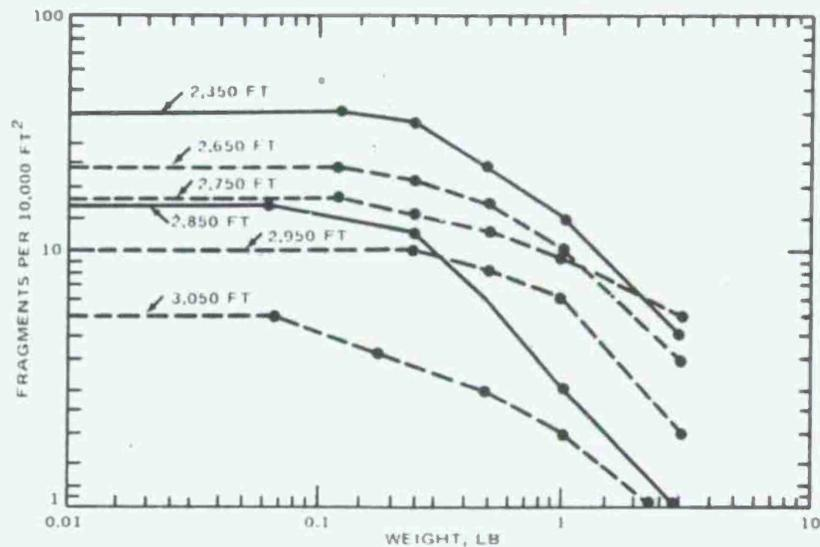
FIG. 53. Cumulative Number of Fragments per 10,000 ft<sup>2</sup> Versus Weight in Pounds for Various Northwesterly Distances From the Donor Magazine (Hand Pickup).
