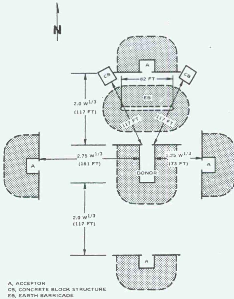
FIG. 1. Layout of Test Structures for ESKIMO I Magazine Separation Test.
