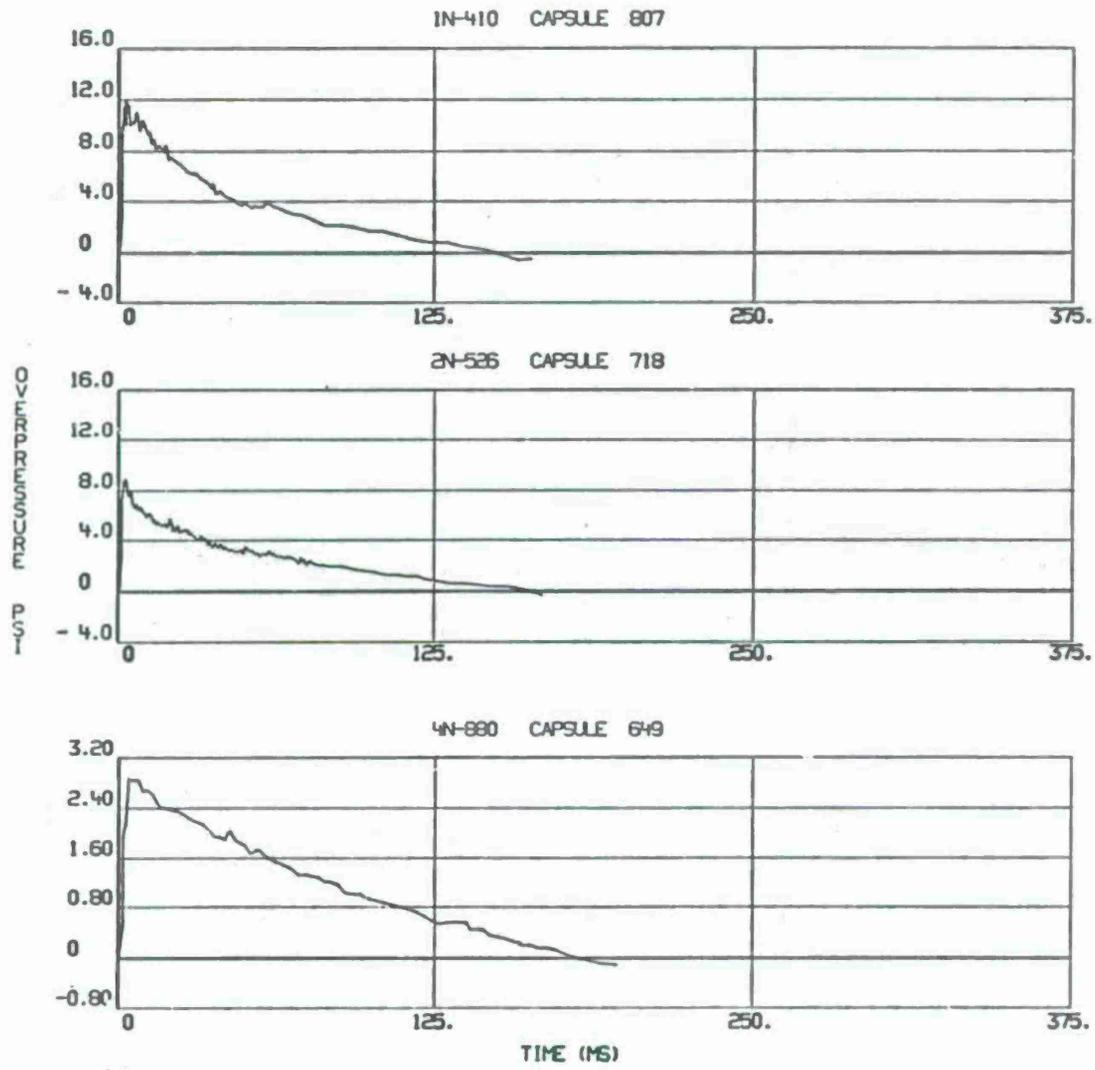
FIG. 70. Data Plots for BRL Gauges 1N, 2N, and 4N.
