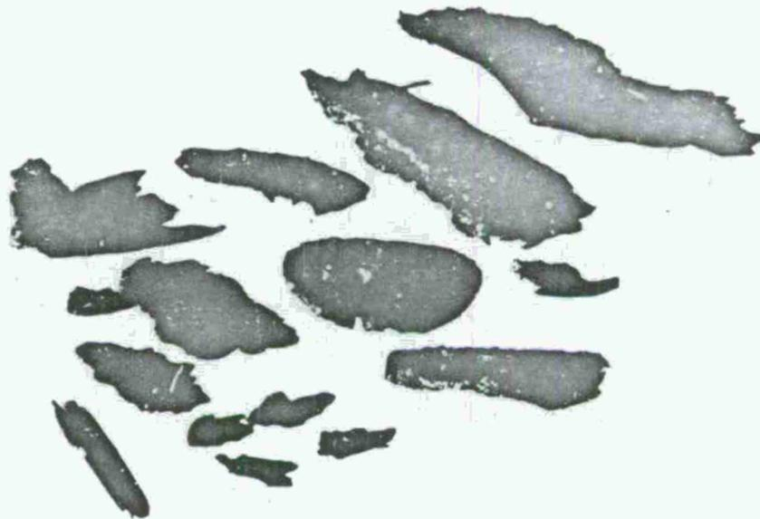
FIG. 48. Projectile Fragments Found at Site of B-29 Aircraft. The largest fragment shown here weighed 10 pounds.
