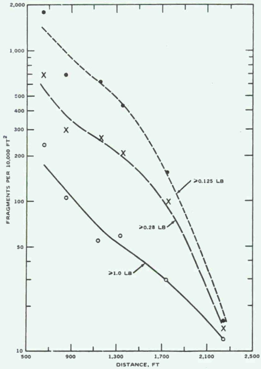
FIG. 64. Number of Fragments per 10,000 ft<sup>2</sup> Versus Distance West of Donor Magazine (Magnetic Pickup).
