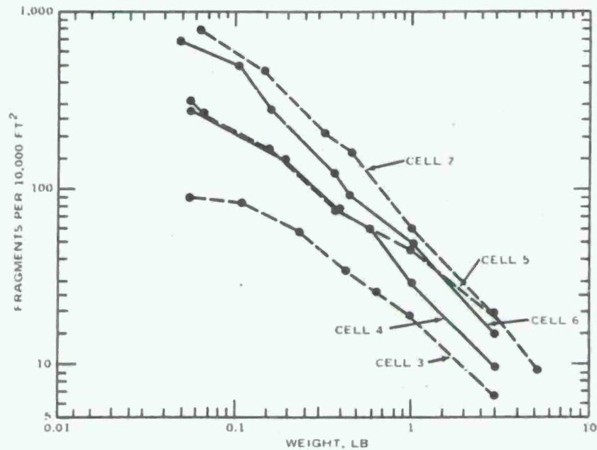
FIG. 51. Cumulative Number of fragments per 10,000 ft<sup>2</sup> Versus Weight in Pounds for Cells in the South Sector (Magnetic Pickup). Cells 1 and 2 were too soft for the truck to operate in.
