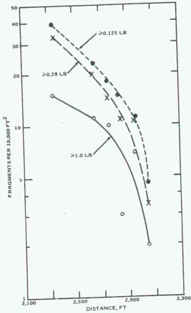
FIG. 59. Number of Fragments per 10,000 ft<sup>2</sup> Versus Distance Northwest of Donor Magazine (Hand Pickup).
