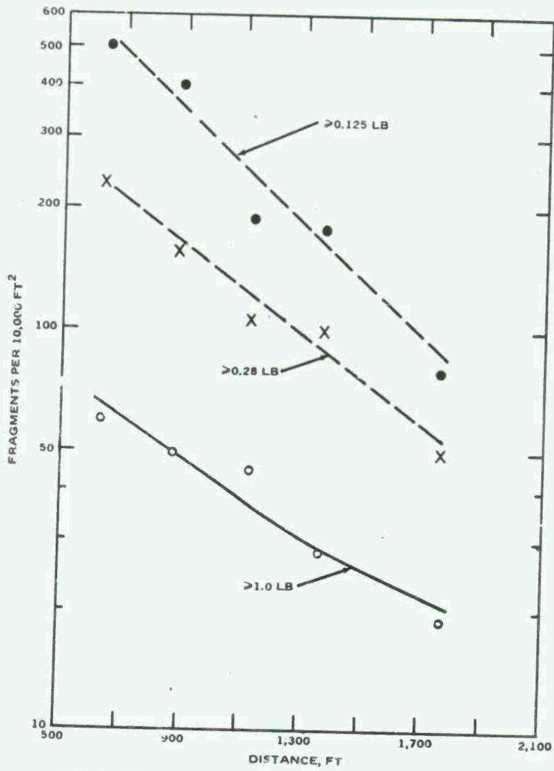
FIG. 60. Number of Fragments per 10,000 ft<sup>2</sup> Versus Distance South of Donor Magazine (Magnetic Pickup).
