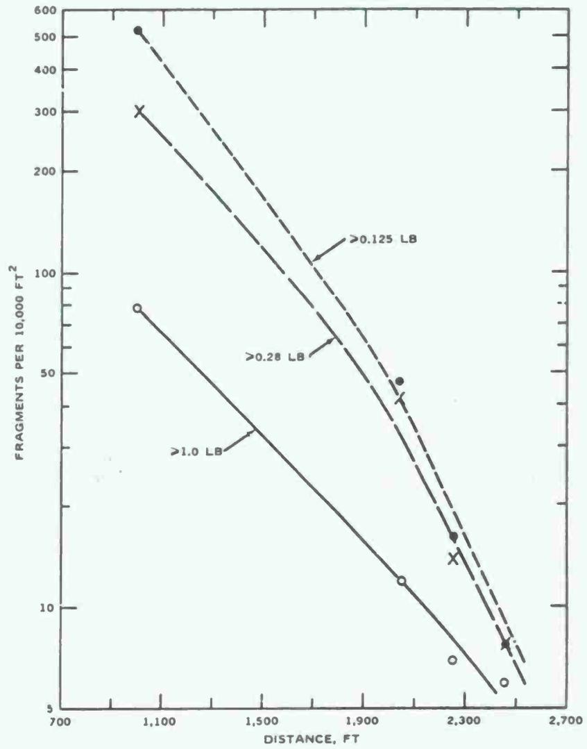
FIG. 61. Number of Fragments per 10,000 ft<sup>2</sup> Versus Distance South of Donor Magazine (Hand Pickup).
