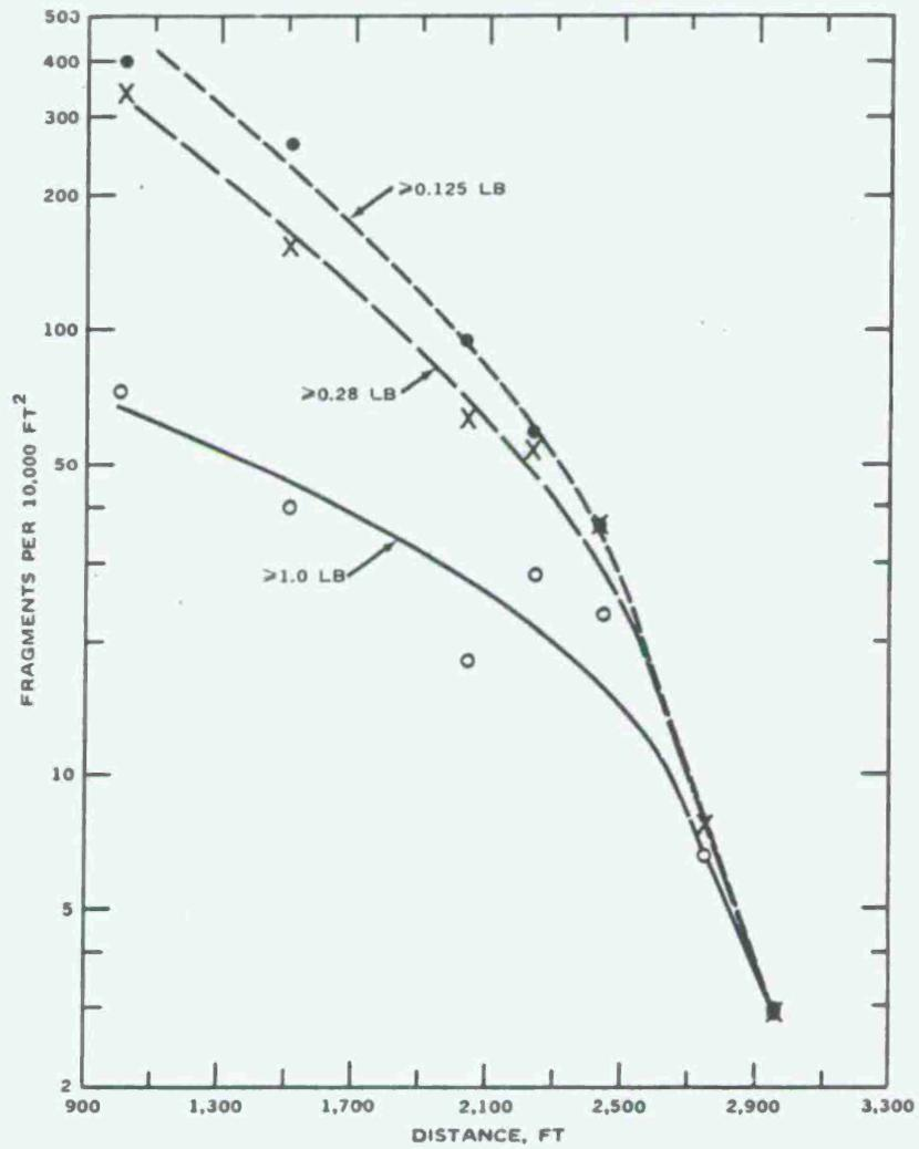
FIG. 65. Number of Fragments per 10,000 ft<sup>2</sup> Versus Distance West of Donor Magazine (Hand Pickup).
