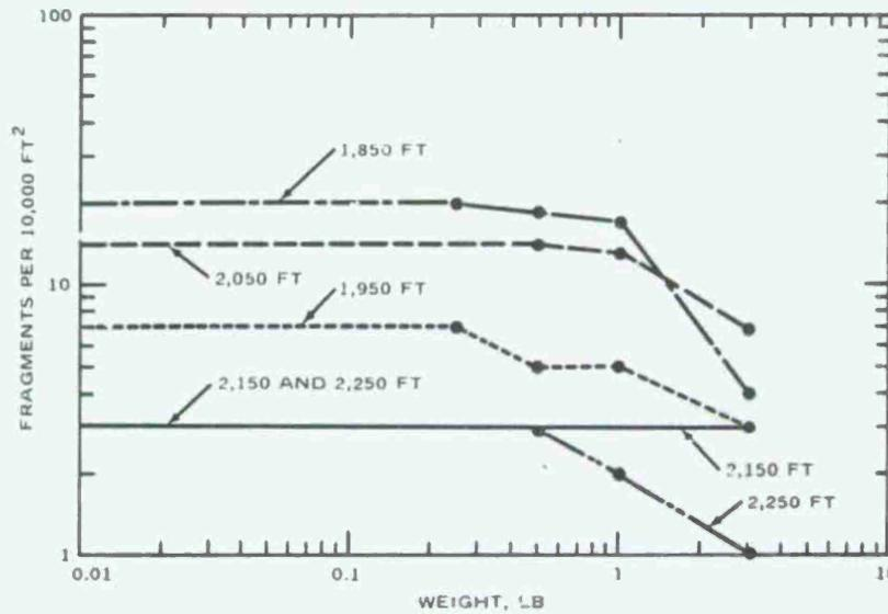
FIG. 57. Cumulative Number of Fragments per 10,000 ft<sup>2</sup> Versus Weight in Pounds for Various Southeasterly Distances From the Donor Magazine (Island Pickup). The 100-by-100-foot area at 2,450 feet was searched, but no fragments were found in it.
