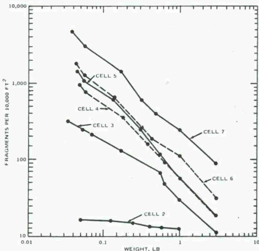
FIG. 52. Cumulative Number of Fragments per 10,000 ft<sup>2</sup> Versus Weight in Pounds for Cells in the West Sector (Magnetic Pickup). Data for Cell 1 is off scale in this figure.
