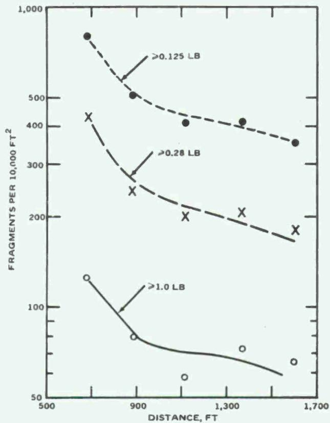
FIG. 62. Number of Fragments per 10,000 ft<sup>2</sup> Versus Distance North of Donor Magazine (Magnetic Pickup).
