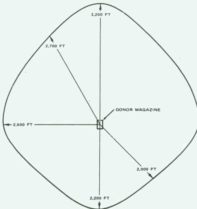
FIG. 66. Limits of Fragment Hazard, Based on Acceptable Density of One Hazardous Fragment per 600 ft<sup>2</sup>. A hazardous fragment is defined as one having kinetic energy  $> 58$  ft-lb.
