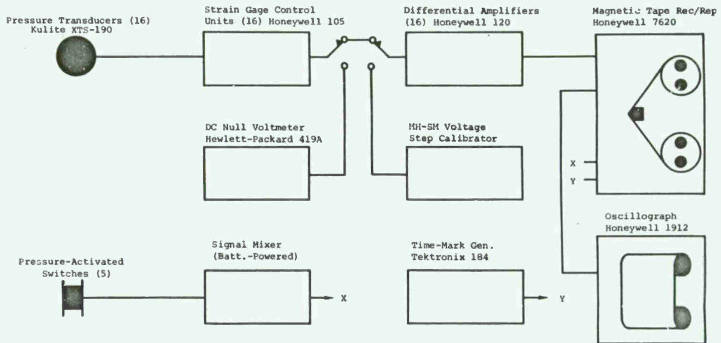
Fig. 5. Block Diagram of Record-Reproduce Instrumentation
