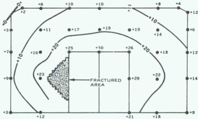
FIG. 79. Movement of Headwall of West Acceptor Igloo. Plus values show movement away from donor magazine; one point (upper left) showed no movement. The units are in hundredths of feet.
