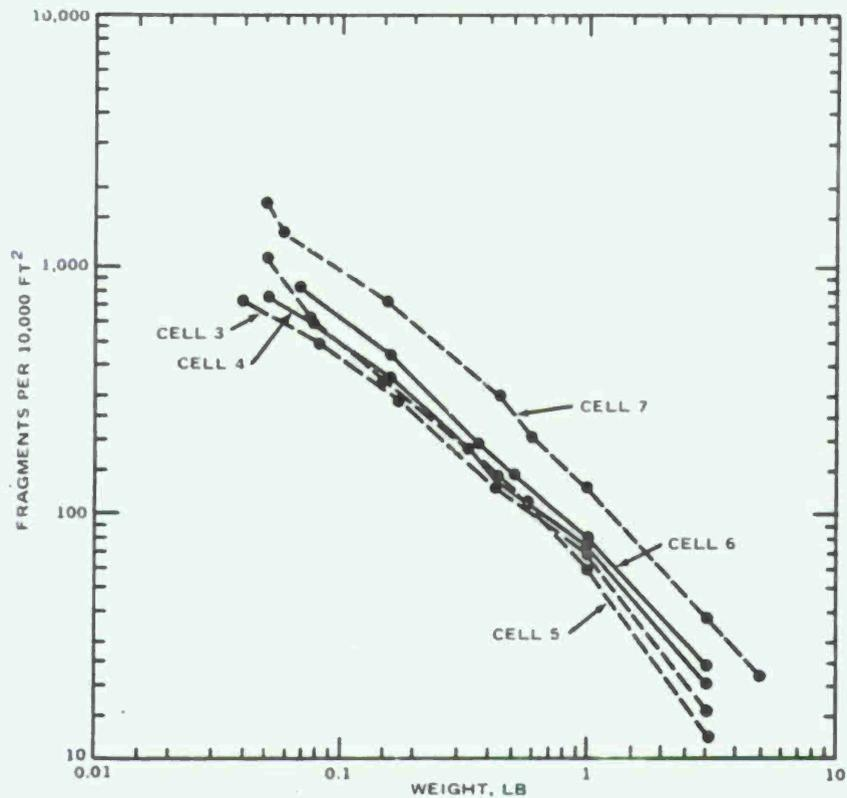
FIG. 50. Cumulative Number of Fragments per 10,000 ft<sup>2</sup> Versus Weight in Pounds for Cells in the North Sector (Magnetic Pickup). Rough, hilly terrain prevented magnetic pickup in Cells 1 and 2.
