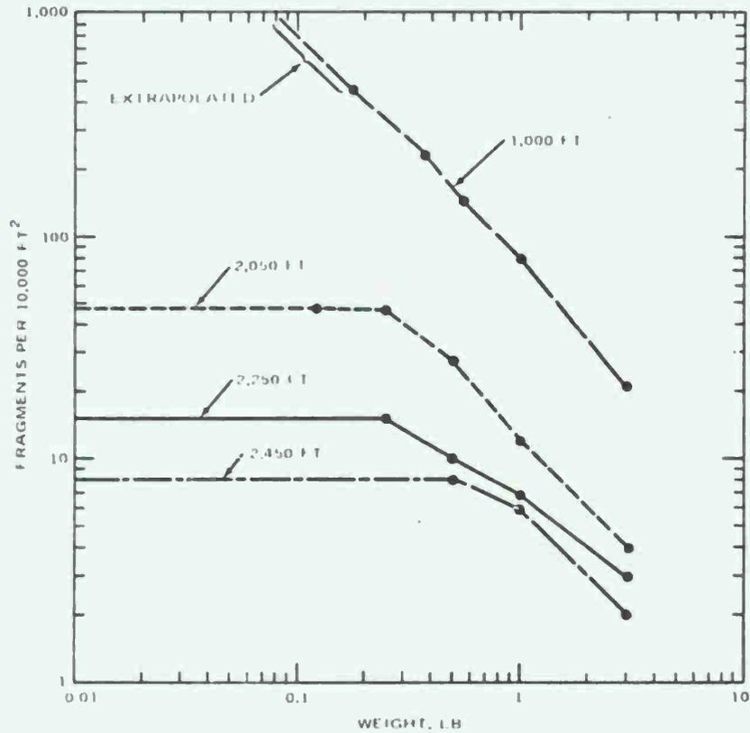
FIG. 56. Cumulative Number of Fragments per 10,000 ft<sup>2</sup> Versus Weight in Pounds for Various Southerly Distances From the Donor Magazine (Hand Pickup). The 1,000-foot curve was extrapolated to obtain a 0.125-pound data point for use in calculations.
