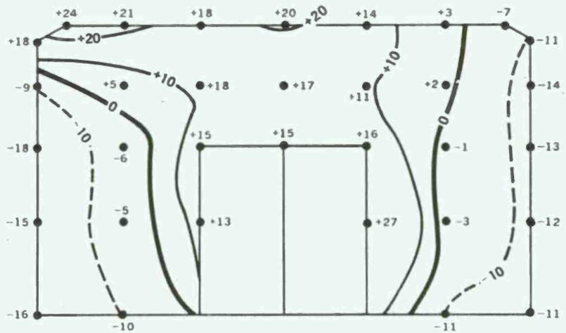
FIG. 78. Movement of Headwall of South Acceptor Igloo. A plus value shows movement away from the donor magazine; a minus value shows movement toward. The units are in hundredths of feet.
