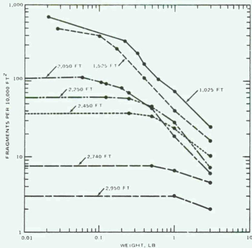
FIG. 54. Cumulative Number of Fragments per 10,000 ft<sup>2</sup> Versus Weight in Pounds for Various Westerly Distances From the Donor Magazine (Hand Pickup).
