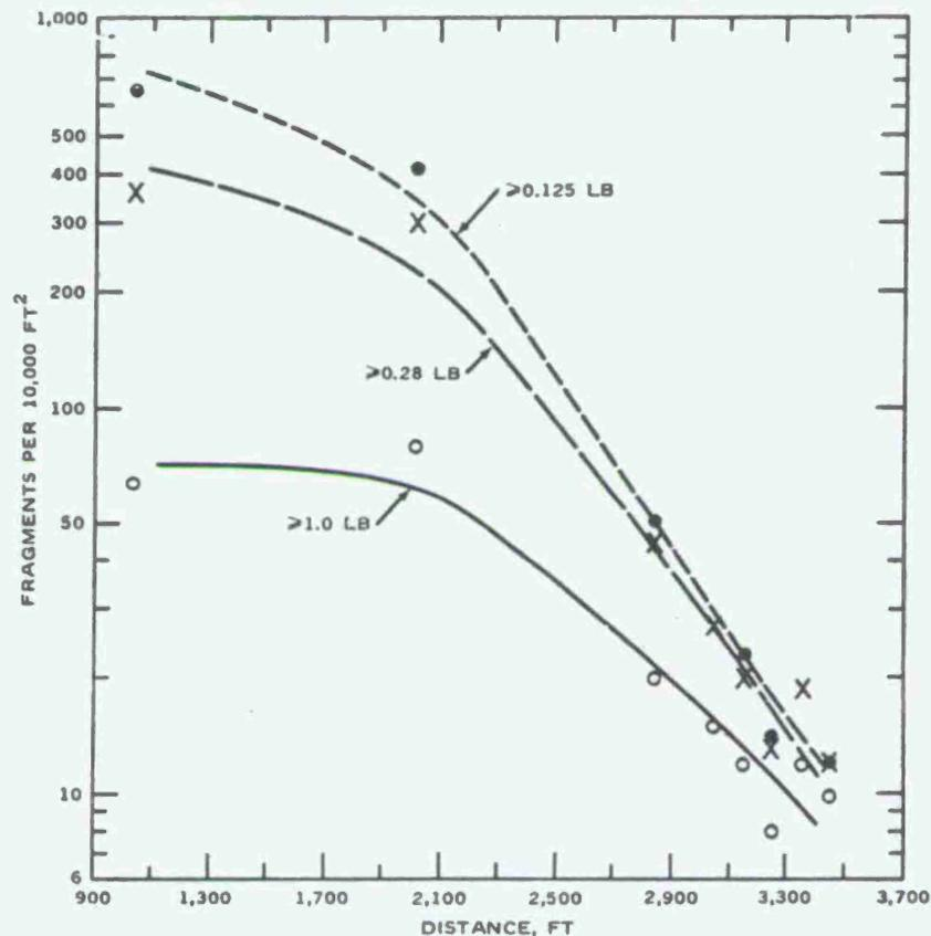
FIG. 63. Number of Fragments per 10,000 ft<sup>2</sup> Versus Distance North of Donor Magazine (Hand Pickup).
