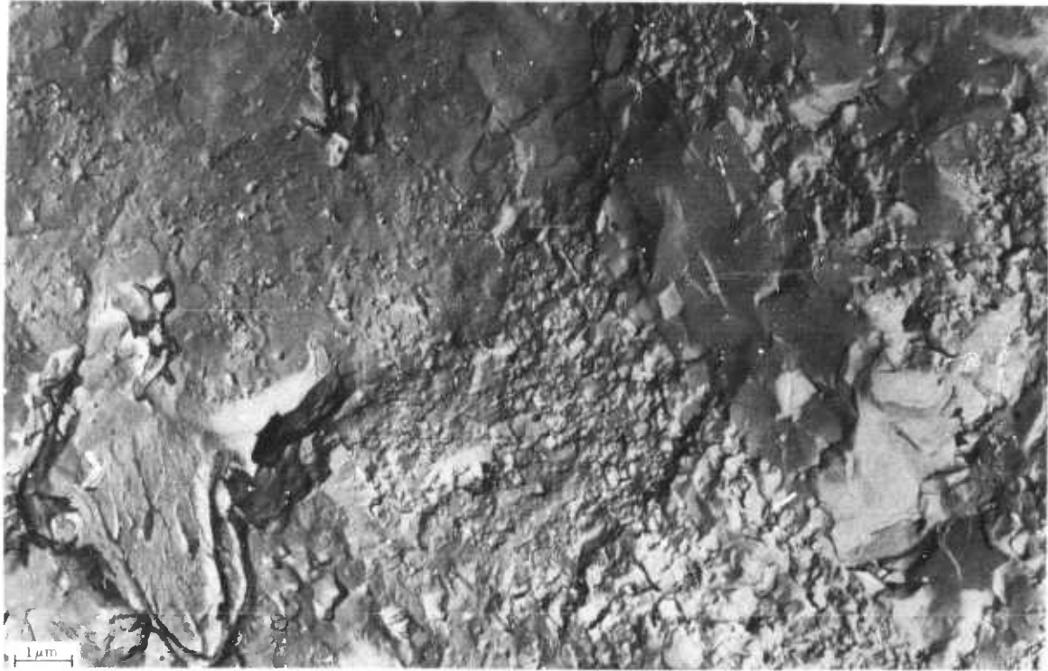
Figure 5.47 — Fracture Surface of Reaction Sintered Si 3 N 4
