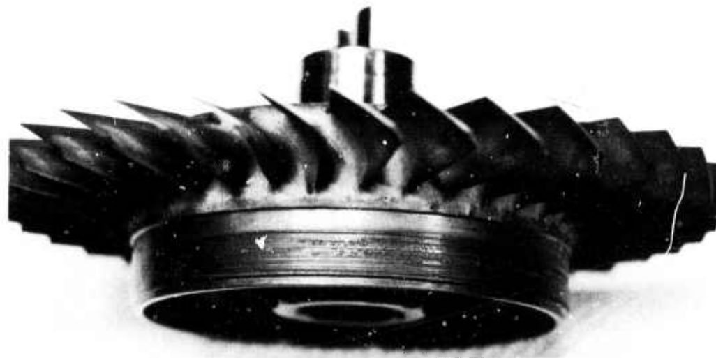
Figure 3.28 — Rotor Showing Rubbed Area of Rim
