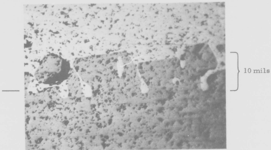
Figure 11(a) Microscopic Photograph of Cross Section for Run Number 32 (88 X). Dark is CdTe; light is Te-rich solution. Substrate temperature 795^{\circ}\text{C} , \Delta T = 5^{\circ}\text{C} .
