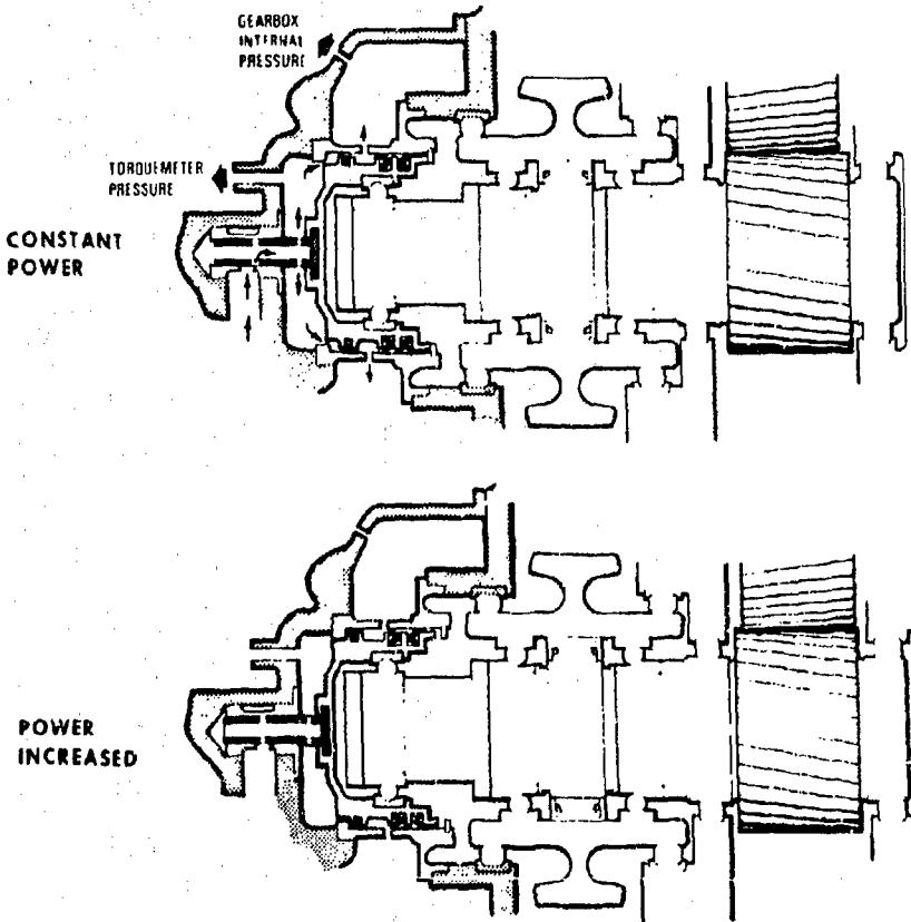
Figure 2. Torquemeter Operation
