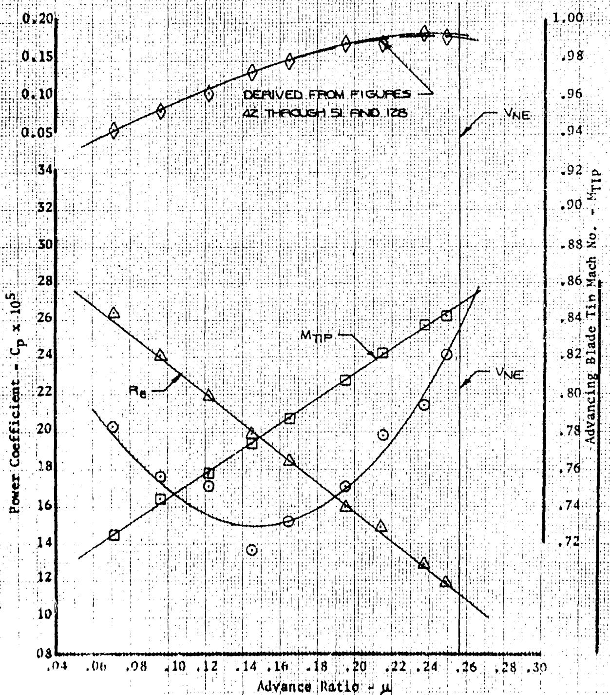
Figure 42. Nondimensional Level Flight Performance
