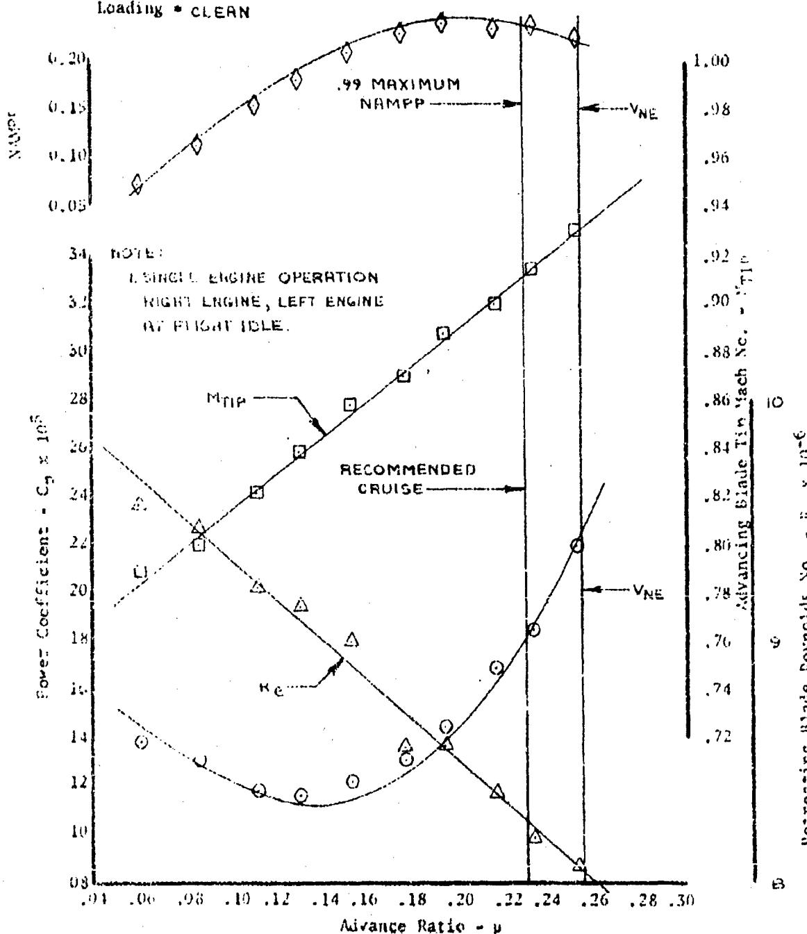
Figure 60. Nondimensional Level Flight Performance
