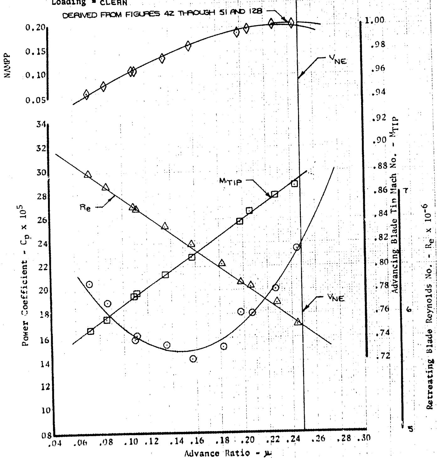
Figure 53. Nondimensional Level Flight Performance
