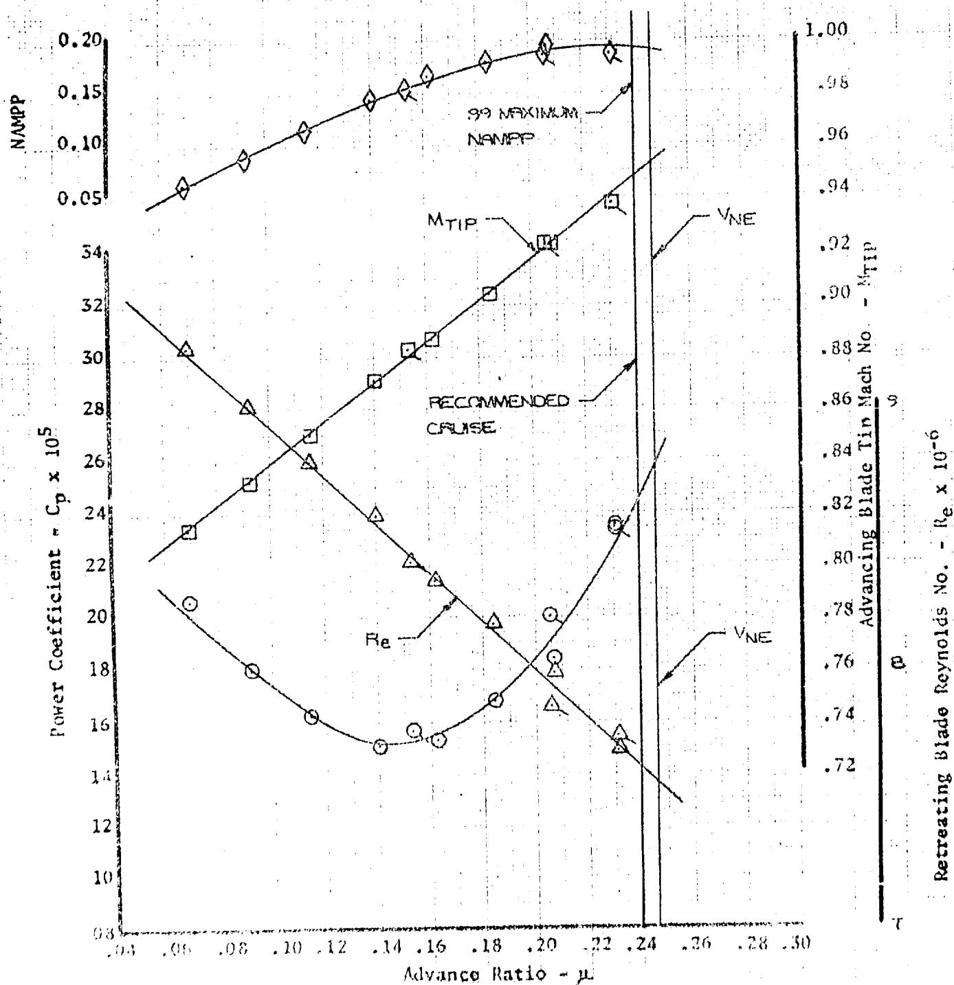
Figure 61. Nondimensional Level Flight Performance
