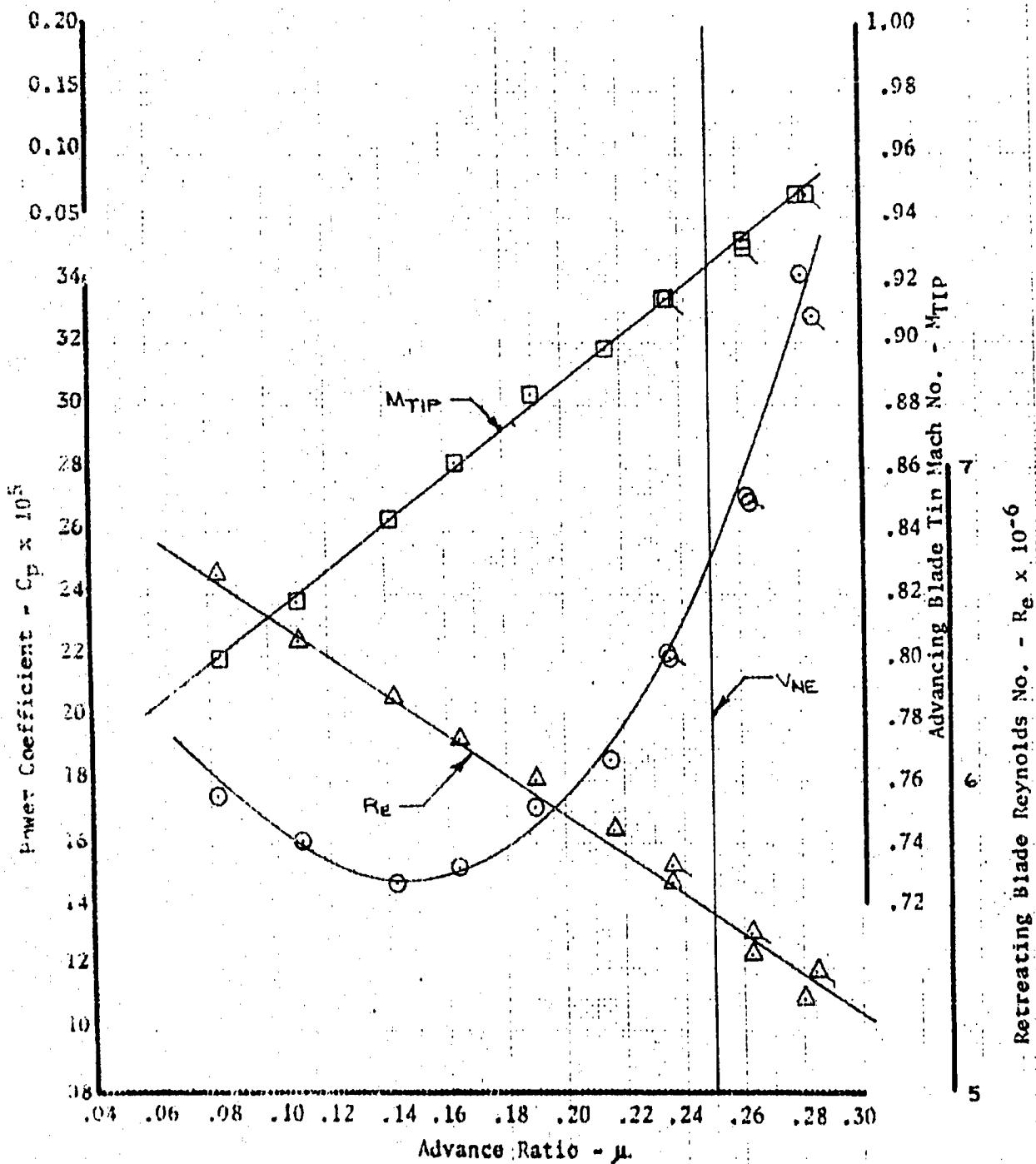
Figure 79. Nondimensional Level Flight Performance
