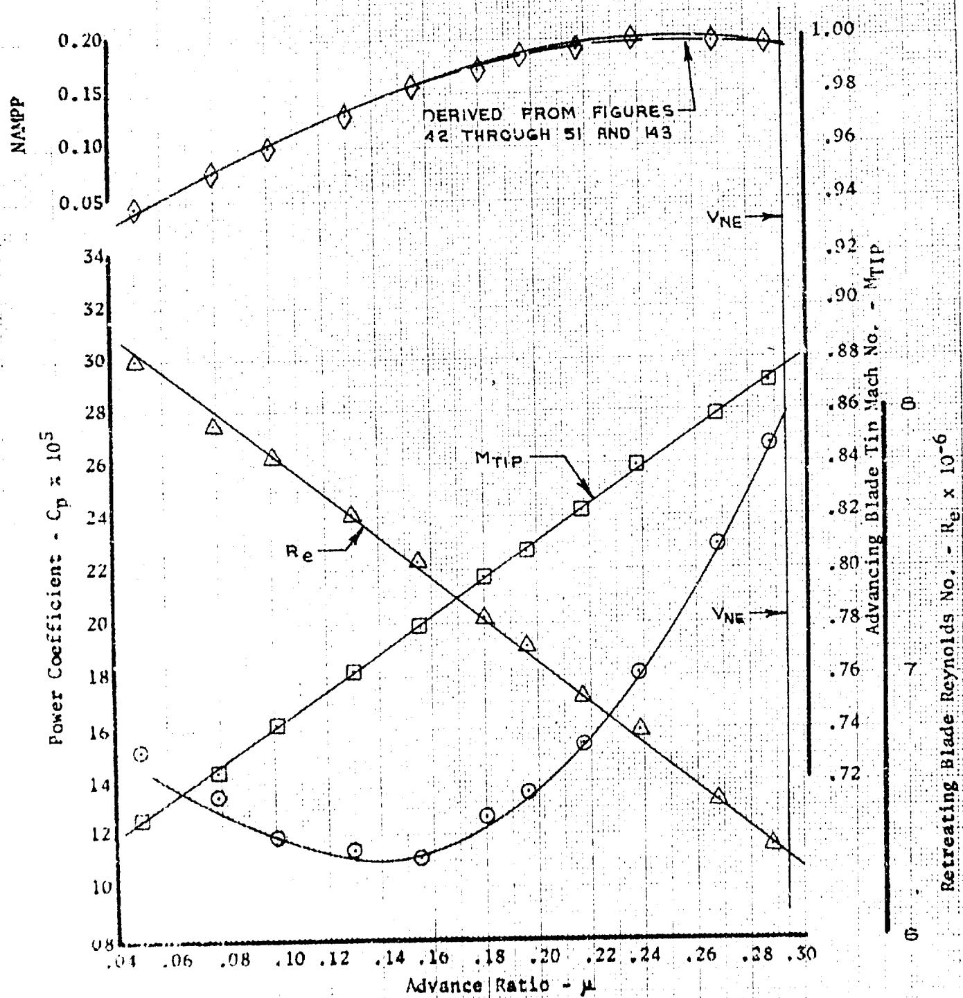
Figure 56. Nondimensional Level Flight Performance
