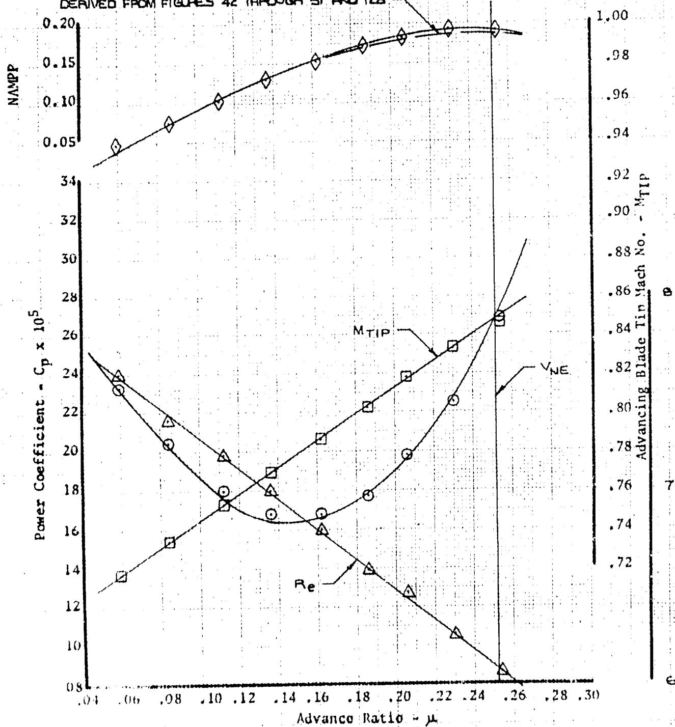
Figure 90. Nondimensional Level Flight Performance
