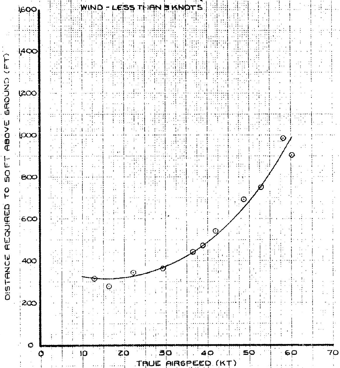
50 FIGURE 35 TAKEOFF DISTANCE REQUIRED TO CLEAR A 50-FT OBSTACLE
