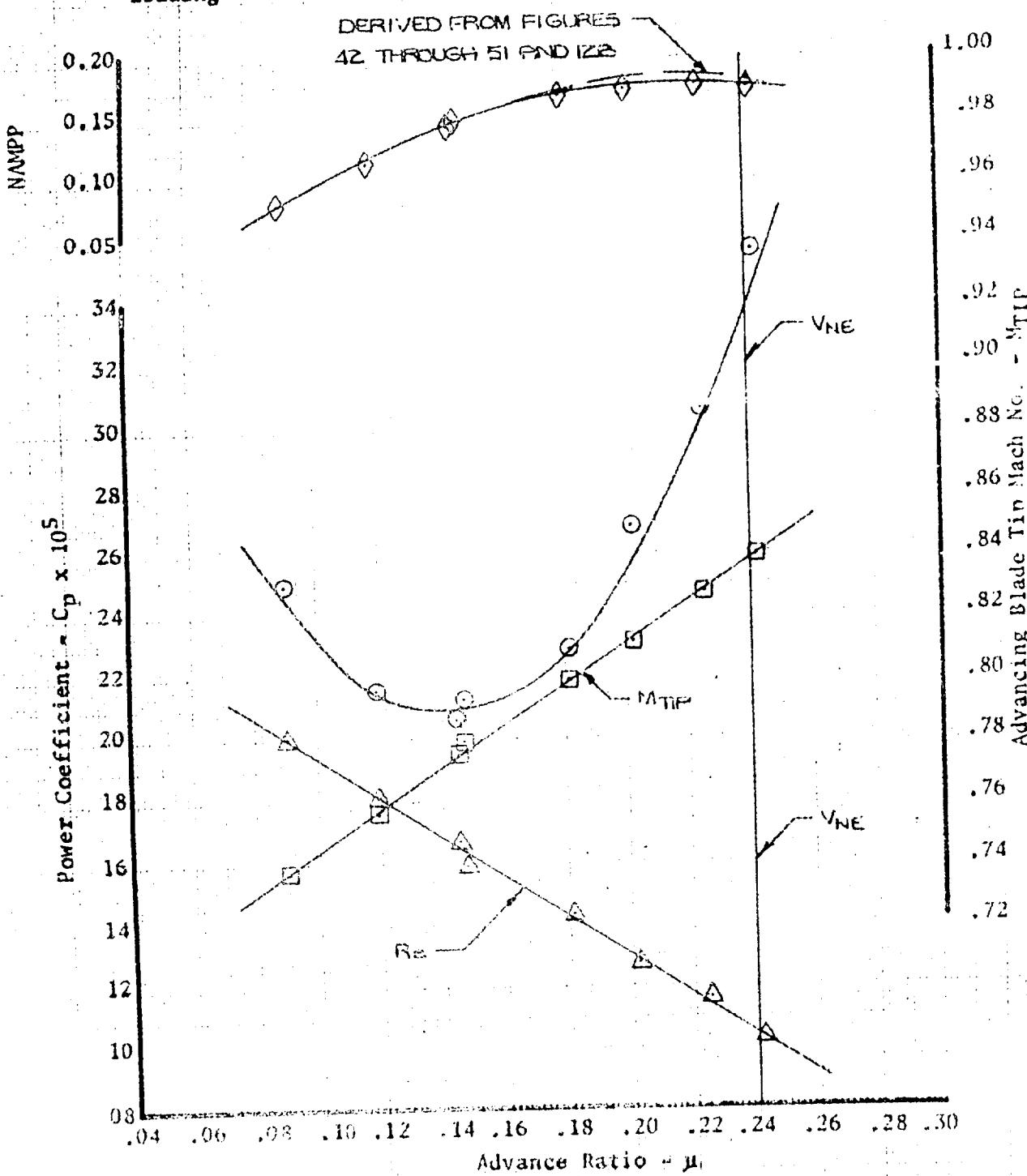
Figure 10. Nondimensional Level Flight Performance
