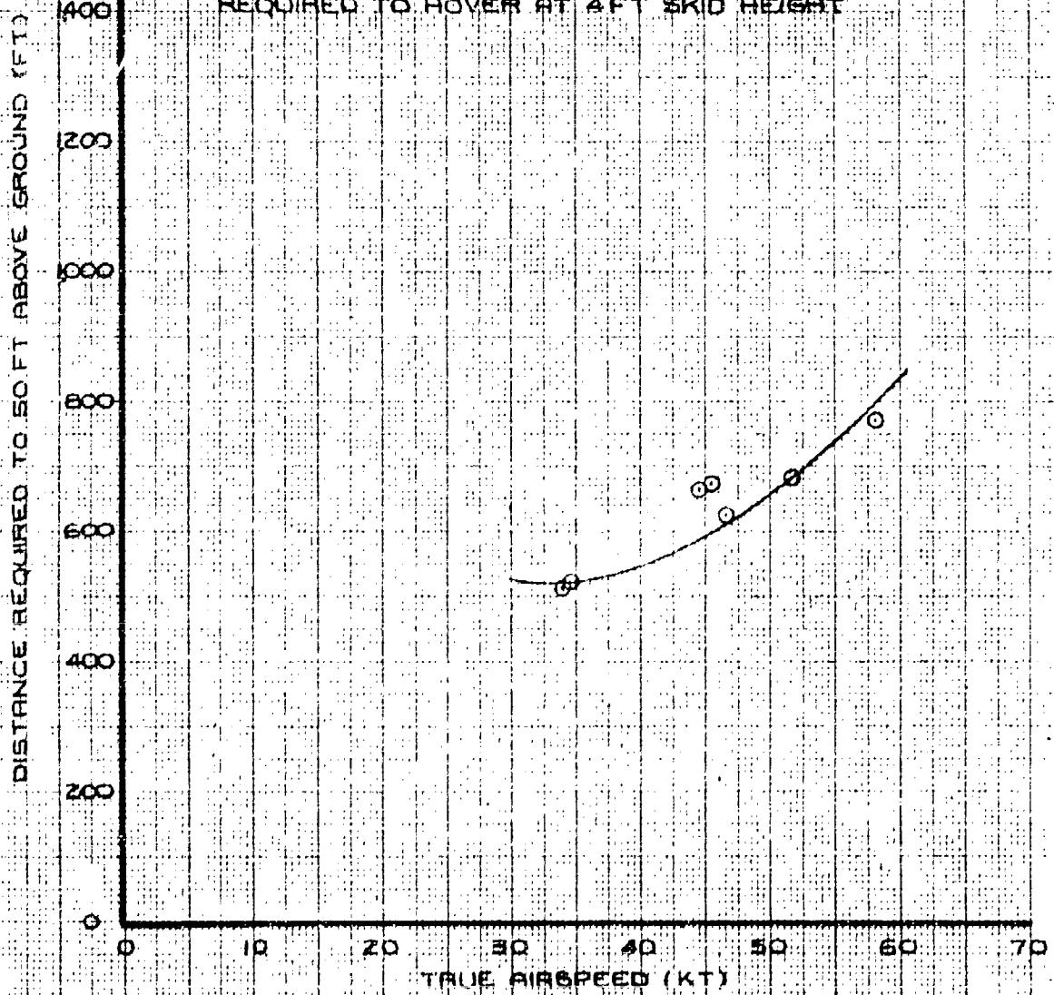
46 FIGURE 31 TAKEOFF DISTANCE REQUIRED TO CLEAR A 50-Ft OBSTACLE
