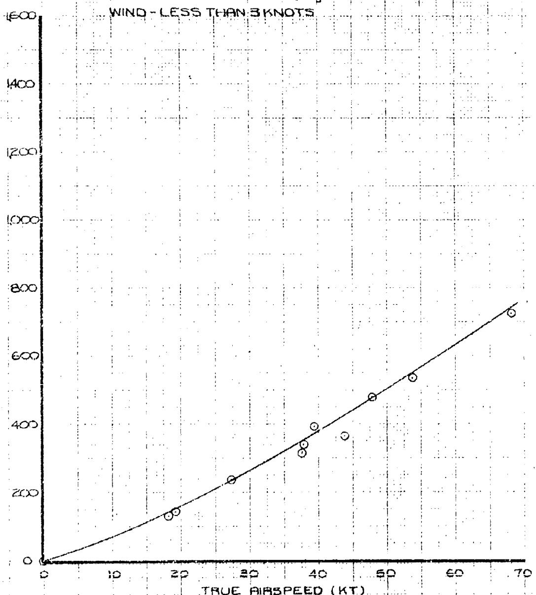
52 FIGURE 37 . TAKEOFF DISTANCE REQUIRED TO CLEAR A SOFT OBSTACLE
