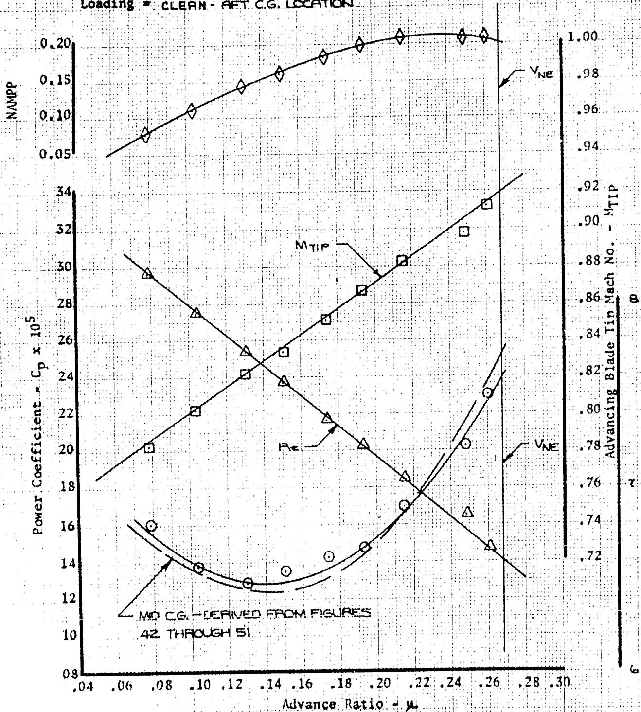
Figure 71. Nondimensional Level Flight Performance
