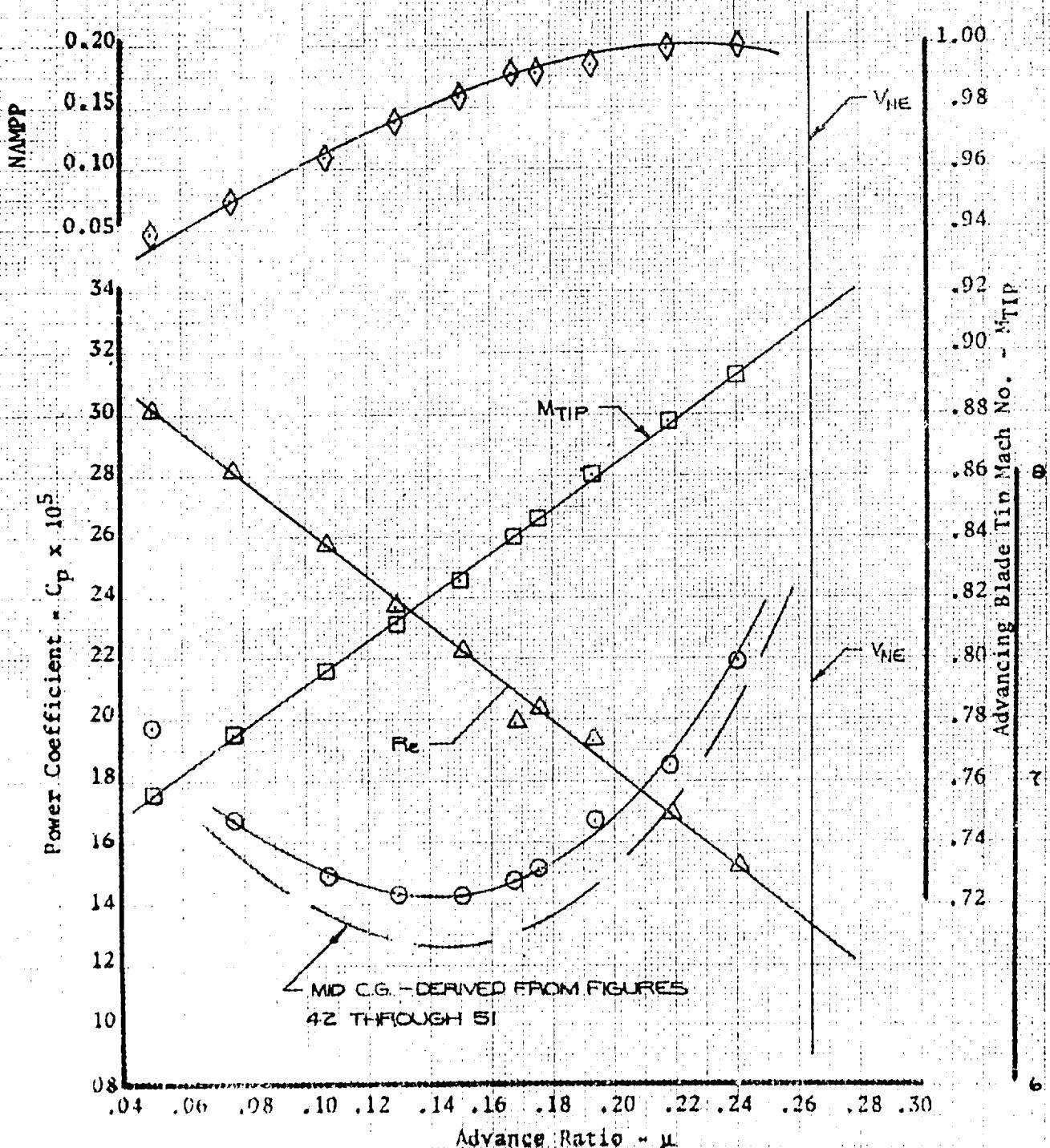
FIGURE 7G Nondimensional Level Flight Performance
