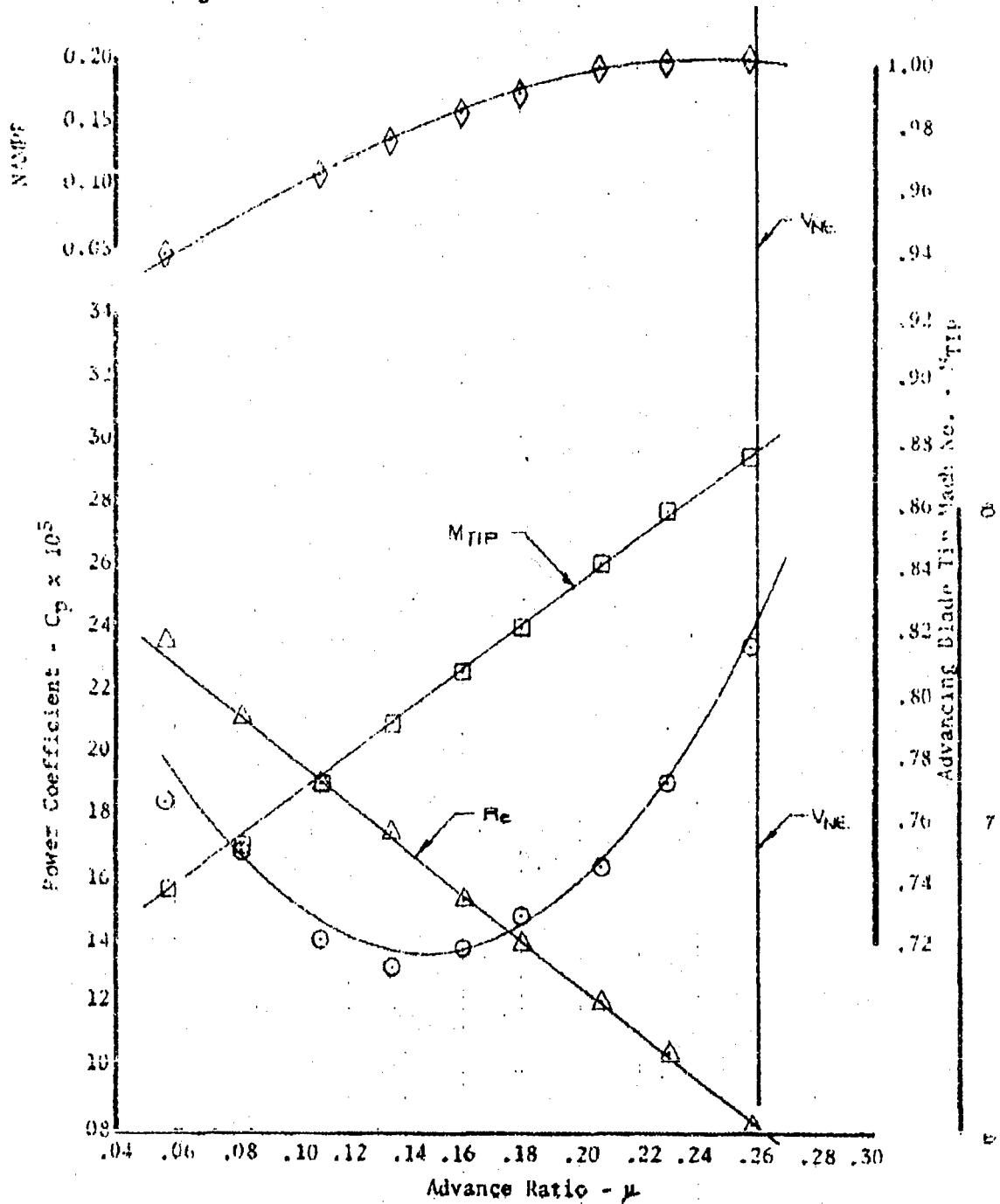
Figure 76. Nondimensional Level Flight Performance
