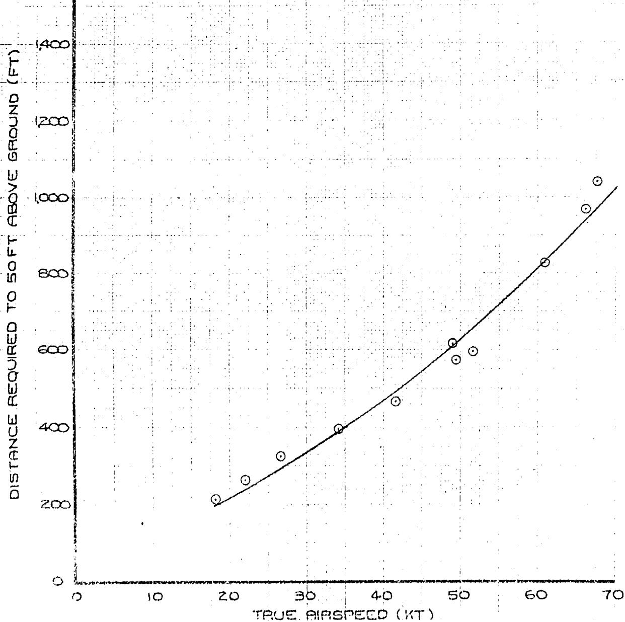
36 FIGURE 21 TAKEOFF DISTANCE REQUIRED TO CLEAR A 50-Ft OBSTACLE
