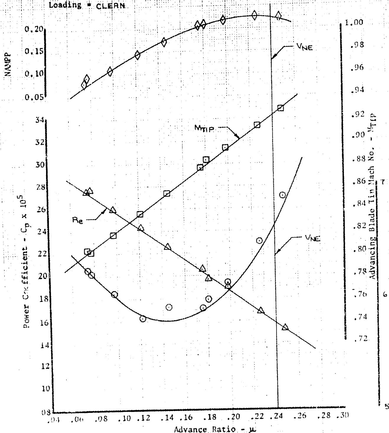
Figure 88. Nondimensional Level Flight Performance
