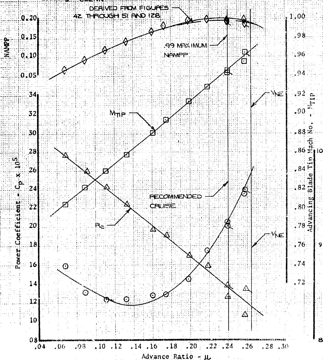
Figure 62. Nondimensional Level Flight Performance
