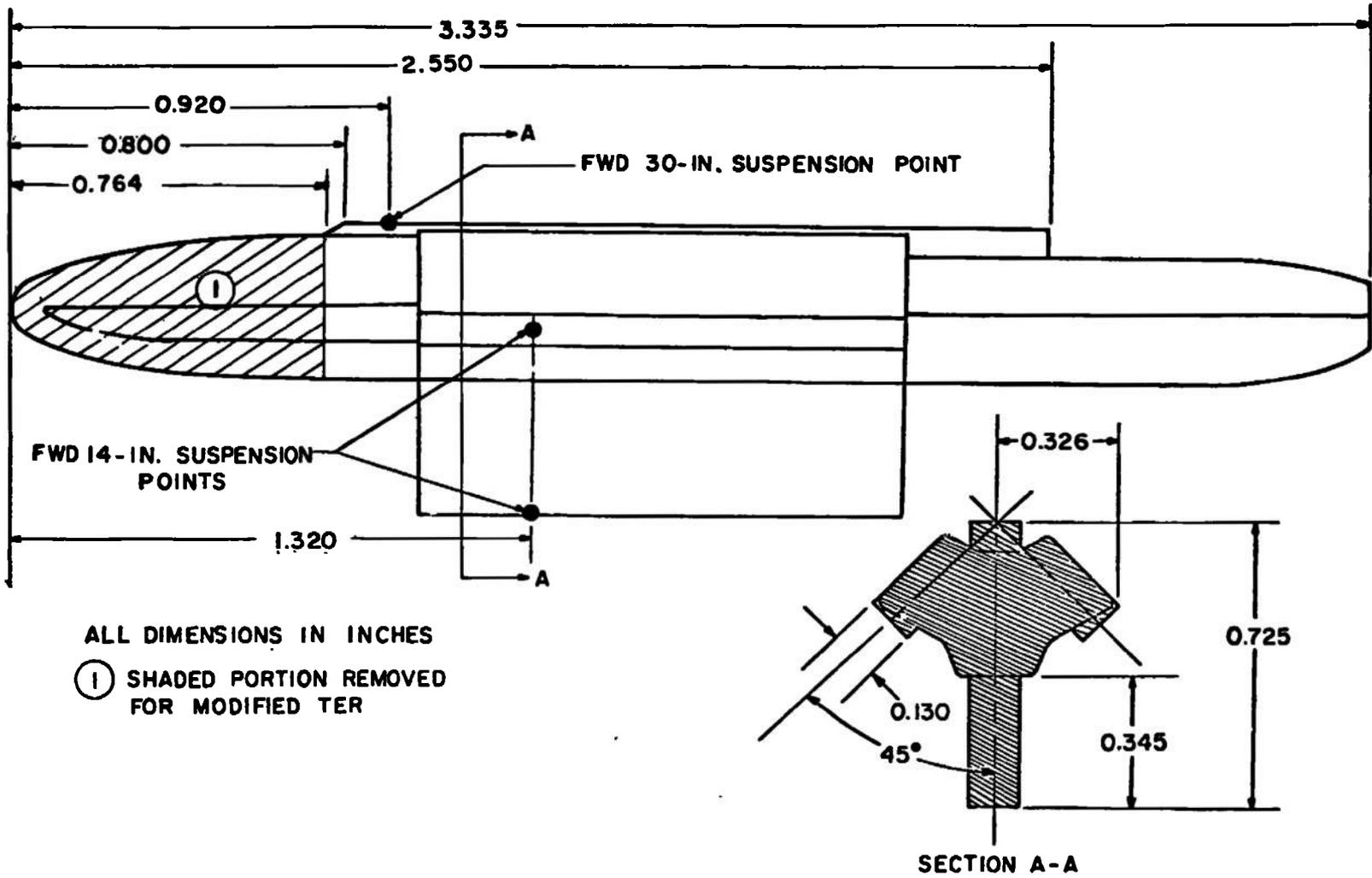
Fig. 6 Details and Dimensions of the TER Models
