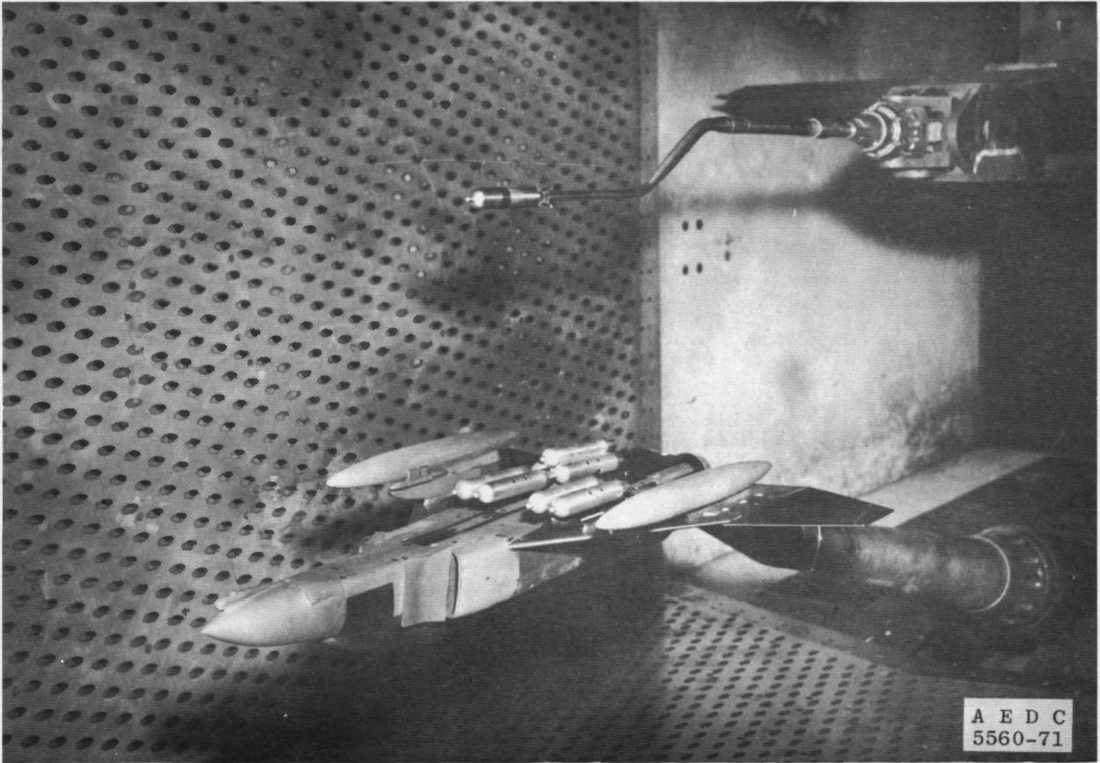
Fig. 10 Photograph Showing a Typical Model Installation for Store Separation Testing
