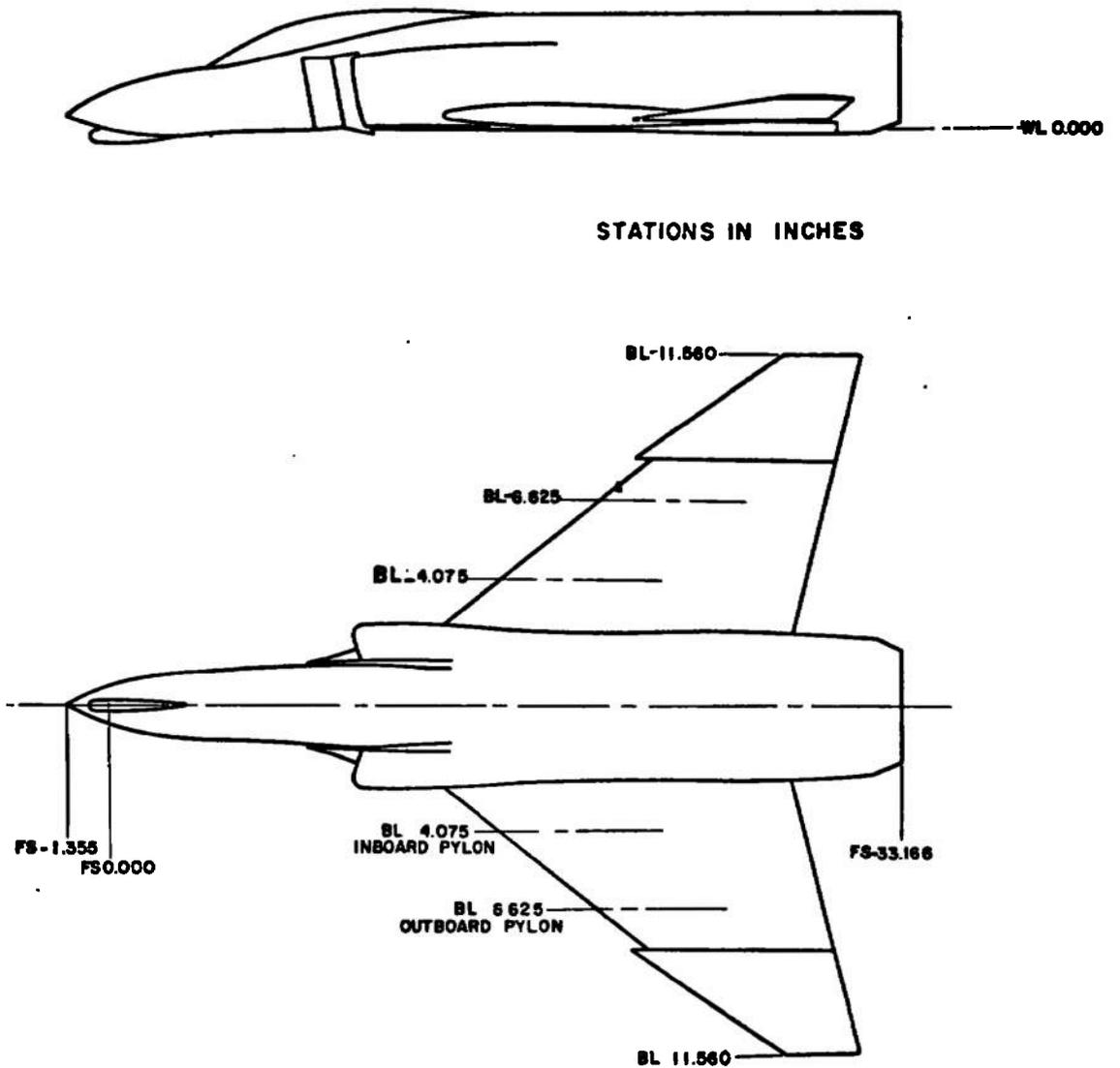
Fig. 3 Sketch of the F-4C Aircraft Model
