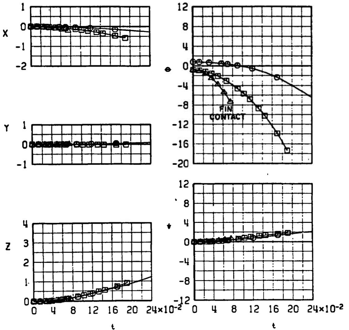
Fig. 17 Trajectory Data for the Ballasted SUU-51B/B from the Standard TER Showing the Effect of Mach Number
