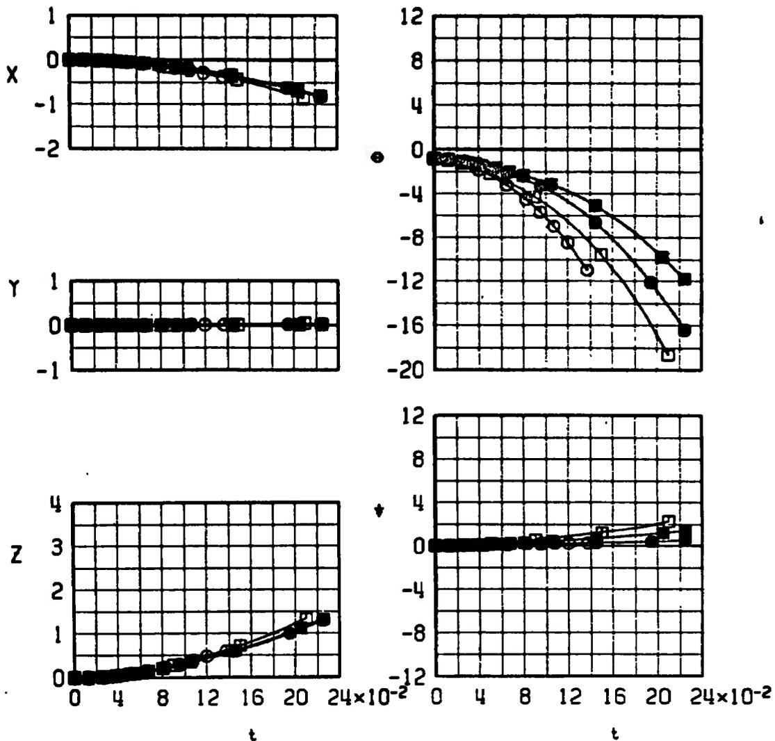
Fig. 19 Trajectory Data Showing the Effect of Store Ballast and TER Geometry with Single Ejector, all Stores Shifted 6 in. Forward
