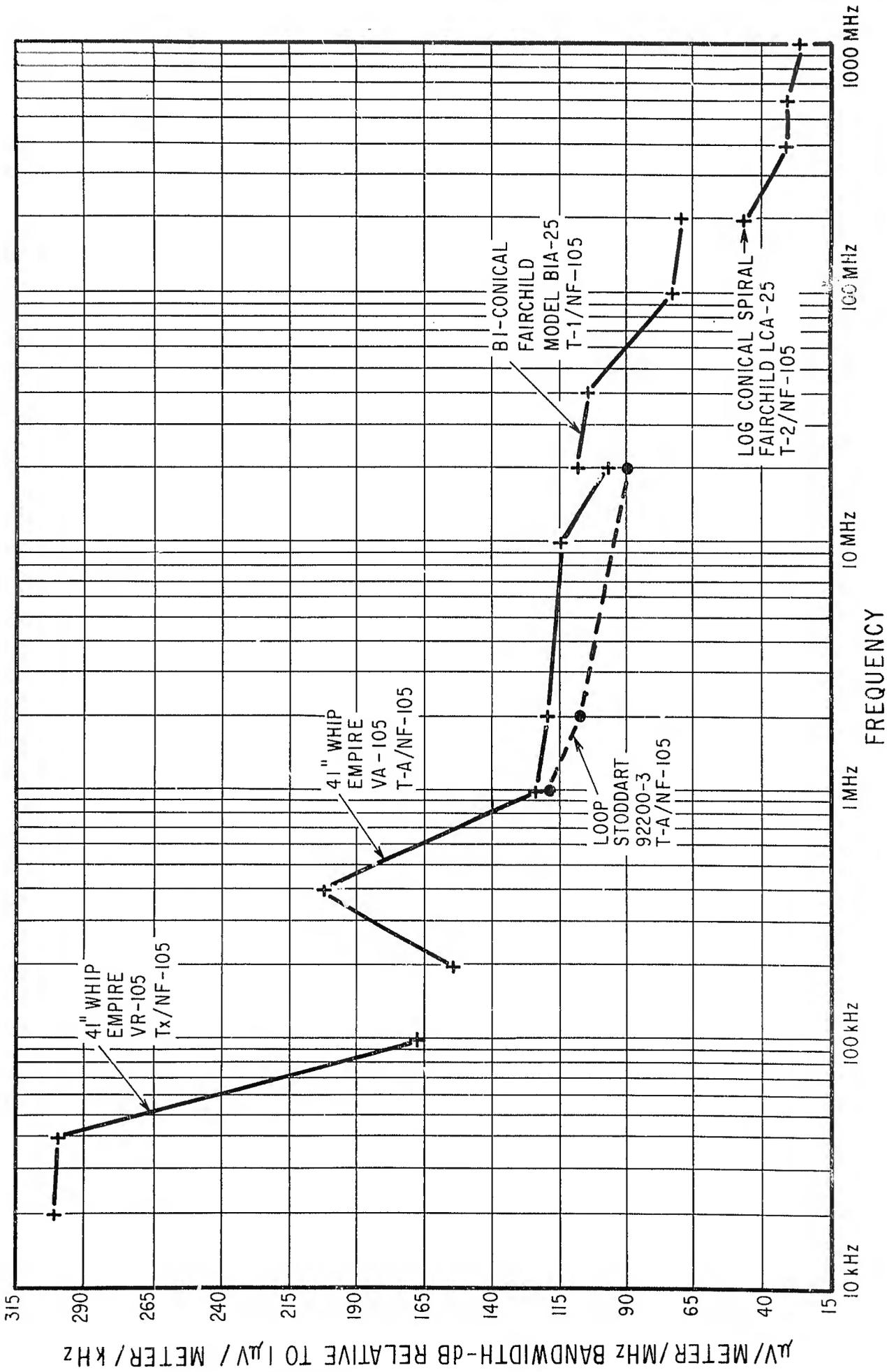
FIGURE 18 - Spectral Density of the Field Associated with a High Voltage Arc
