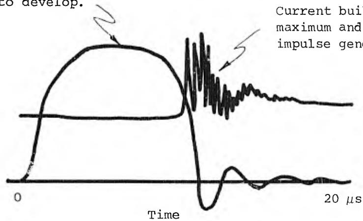
FIGURE 20 Voltage Across, and Current Through, the Four-meter Arc
