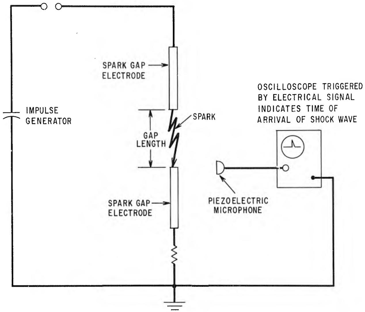
FIGURE 22 - Directly-Coupled Microphone For Measurement of Shock-Wave Arrival Times
