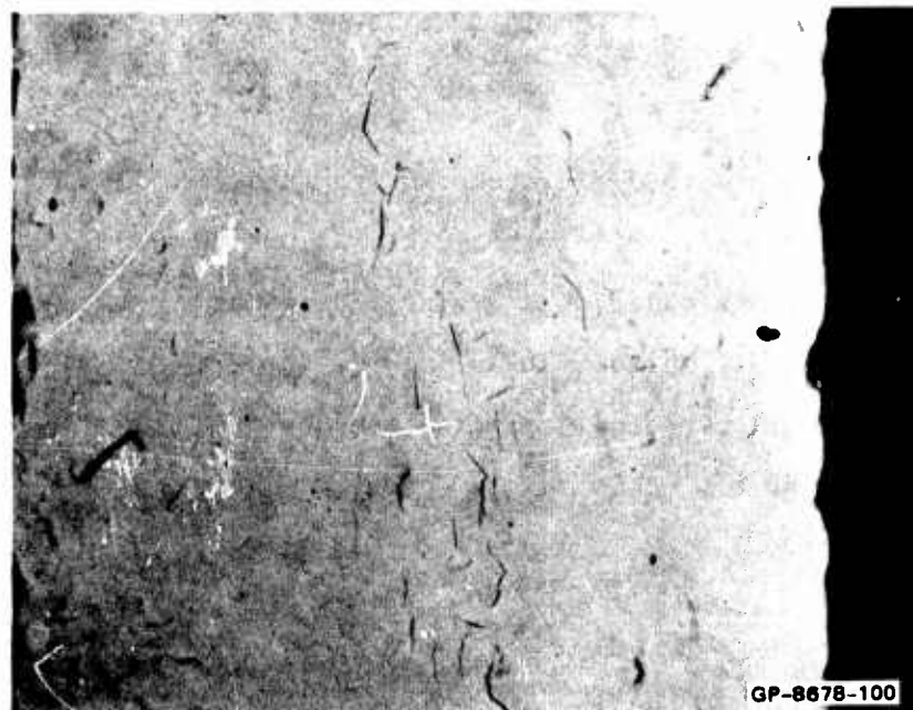
FIG 47 THRESHOLD DAMAGE IN 99.99% PURE IRON
