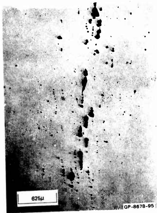
FIGURE 10 SHOCK DAMAGE IN HIGH PURITY ALUMINUM
