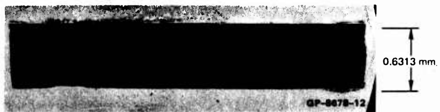
FIGURE 62 DAMAGE OBSERVED IN SHOT S1, A TAPERED FLYER SHOT ON ARMCO IRON
