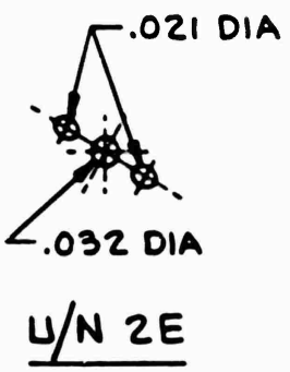
Figure 95. Unit 2D and 2E Triplet, Double-Panel Injector, Injection Element Configurations
