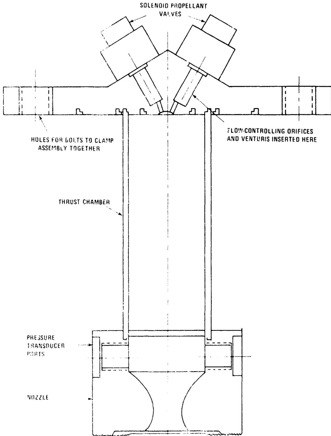
Figure 5. Thruster and Propellant Injection System
